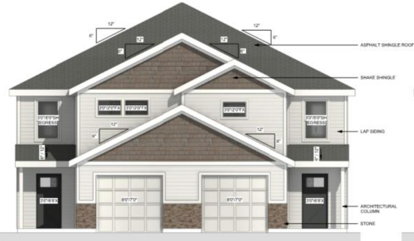
① B2 DUPLEX FRONT ELEVATION 1/4" = 1'-0"
