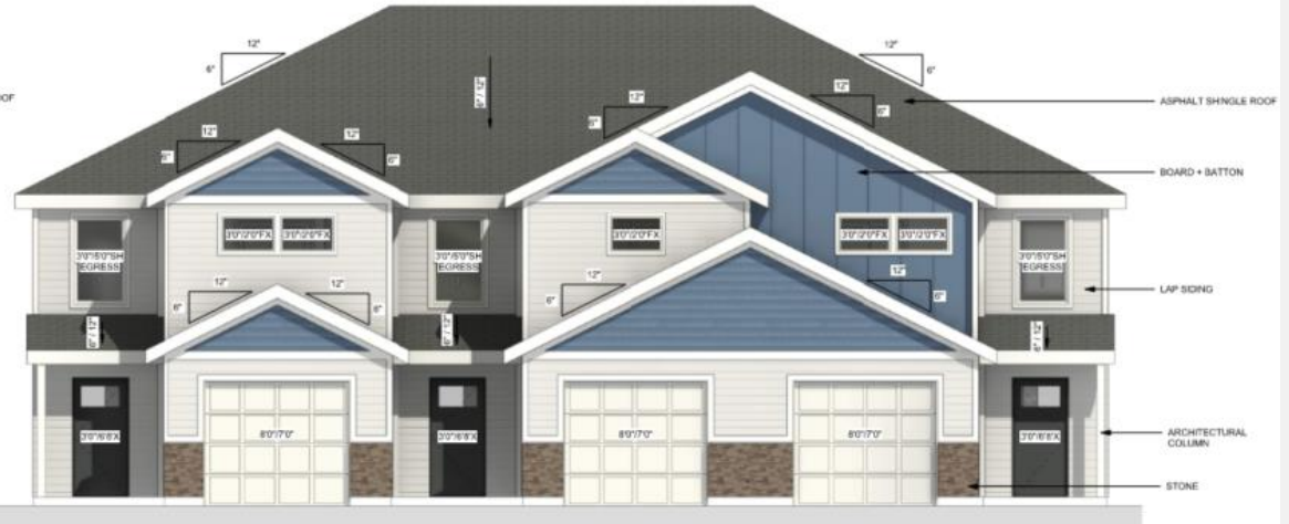
③ B2 TRIPLEX FRONT ELEVATION 1/4" = 1'-0"
