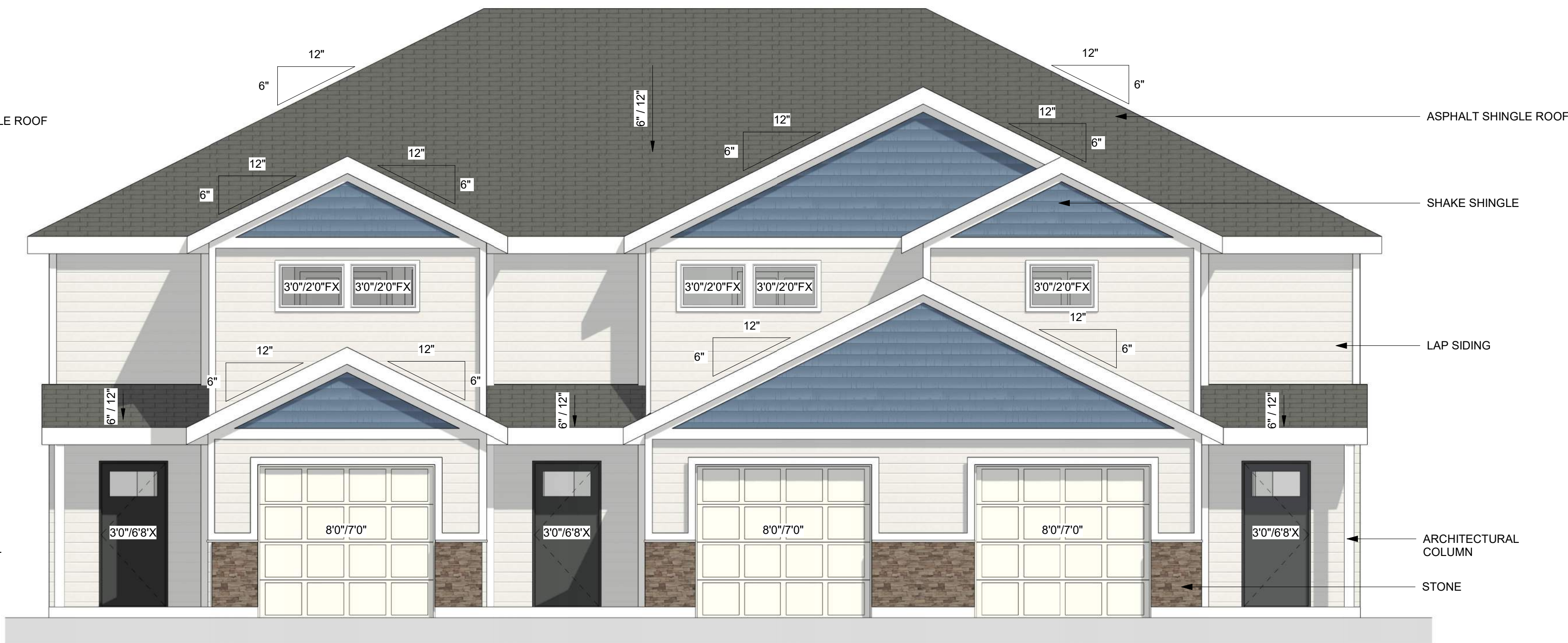
③ A2 TRIPLEX FRONT ELEVATION 1/4" = 1'-0"
