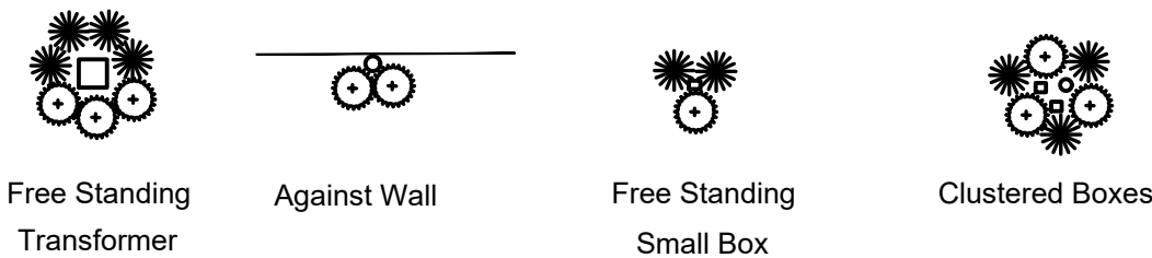
TYPICAL UTILITY BOX SCREENING DETAILS - NTS
