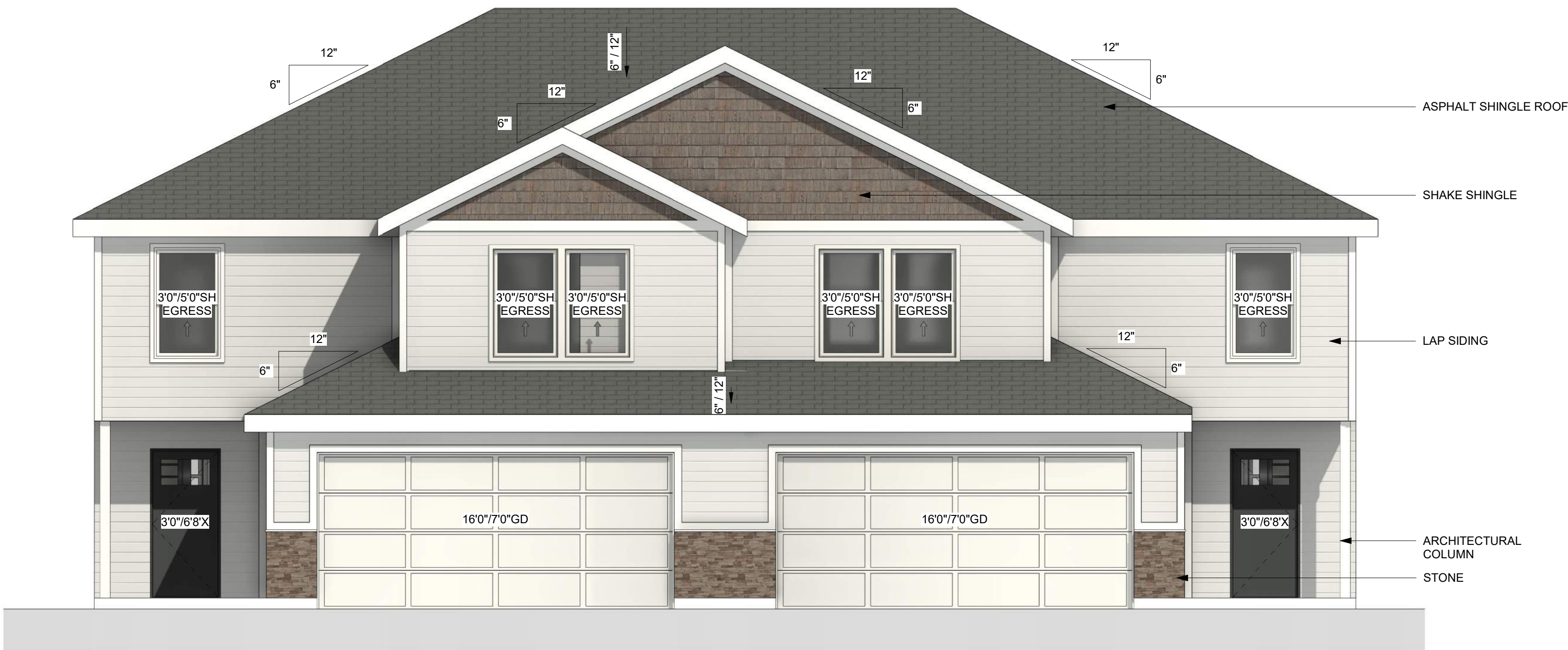
① C2 DUPLEX FRONT ELEVATION 1/4" = 1'-0"
