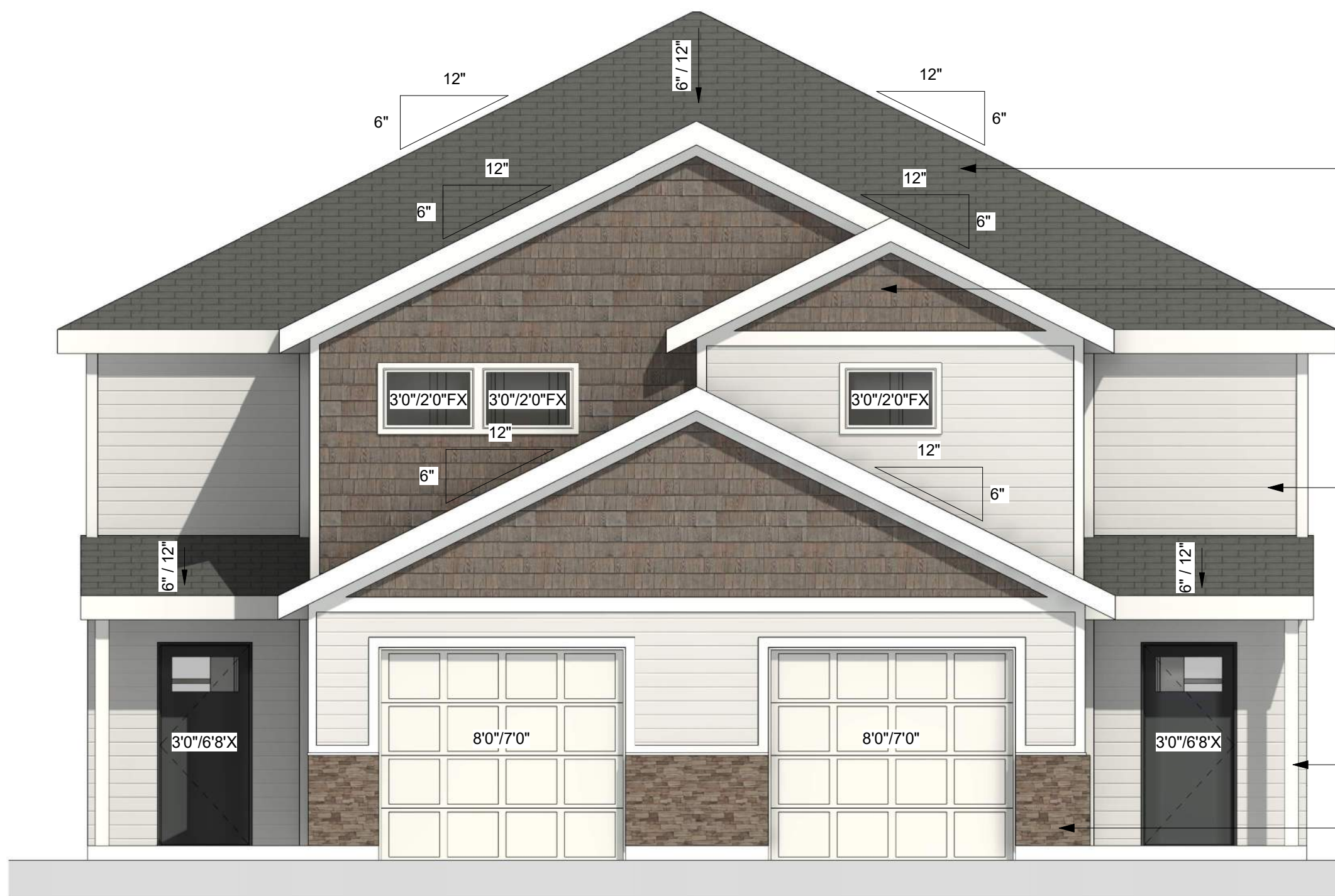
① A2 DUPLEX FRONT ELEVATION 1/4" = 1'-0"
