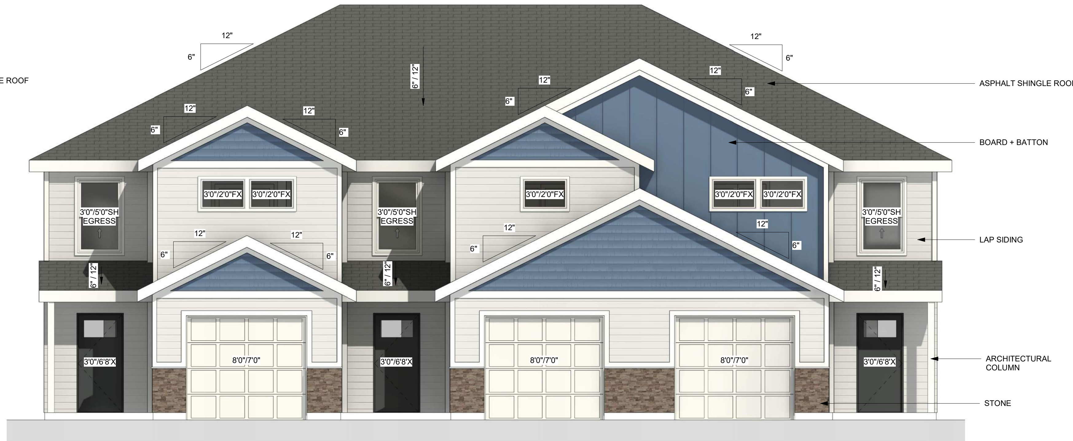
3 B2 TRIPLEX FRONT ELEVATION 1/4" = 1'-0"
