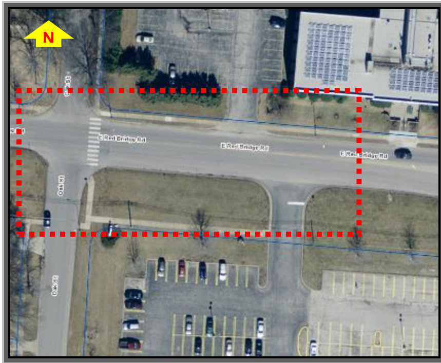
Closely Spaced & Improperly Offset Roadways & Entrances
