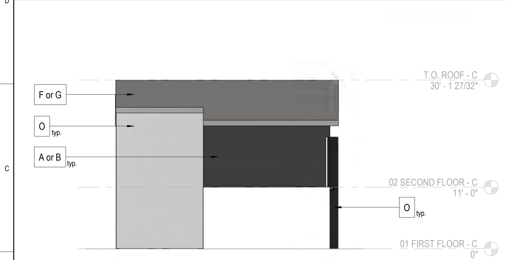
B12 BUILDING C NORTHEAST ELEVATION 1" = 10'-0"
