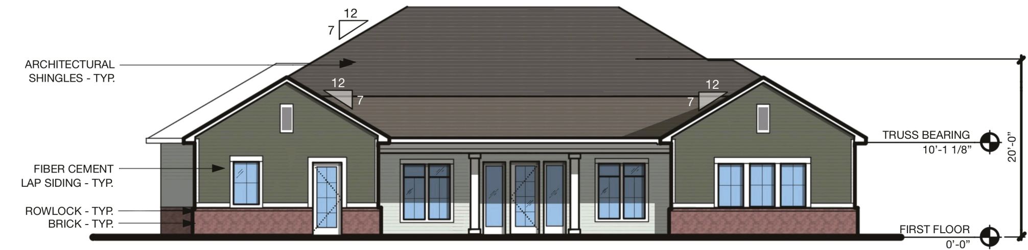
REAR ELEVATION - COMM. BUILDING 3/32"=1'-0" B1
