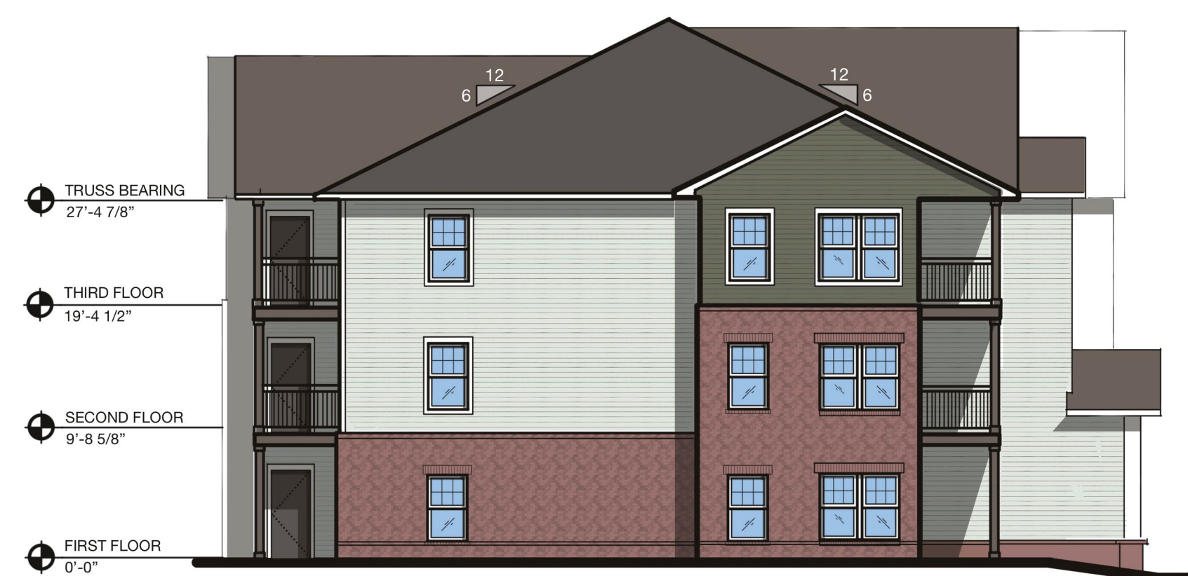
SIDE ELEVATION - ALL 12B6C BLDGS.
