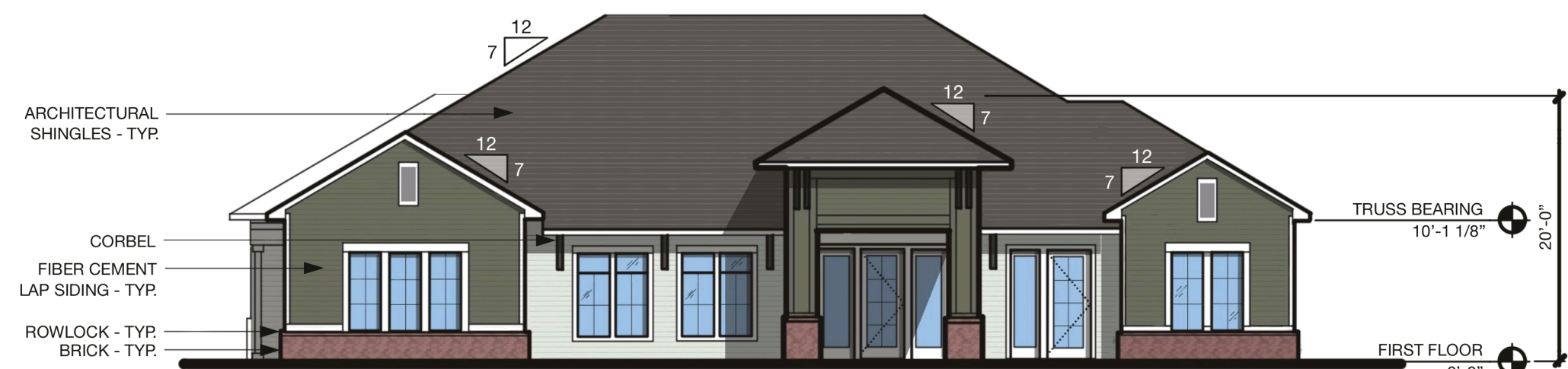
FRONT ELEVATION - COMM. BUILDING 3/32"=1'-0" A1
