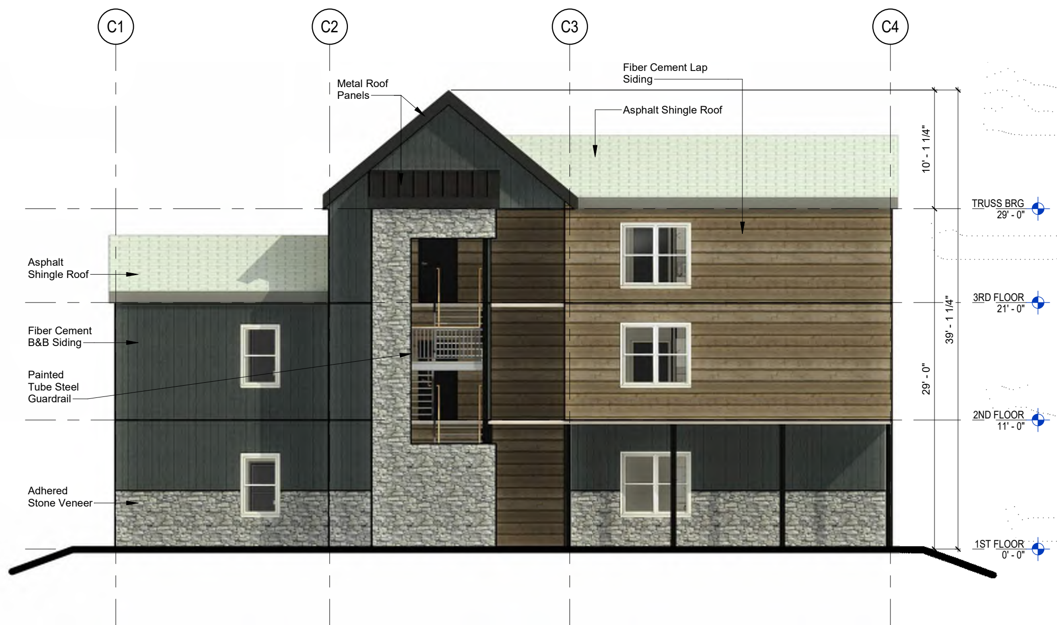
1 SOUTH ELEVATION - BLDG C 1/8" = 1'-0"
