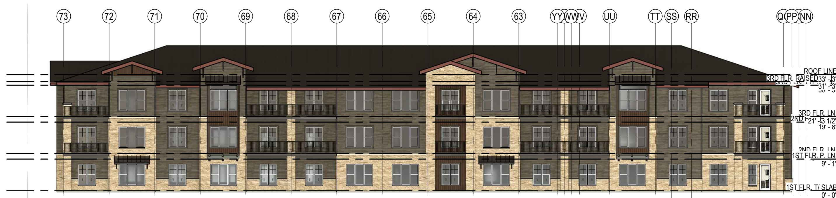
5 EXTERIOR ELEVATION BLDG. 2 - EAST 1/16" = 1'-0"
