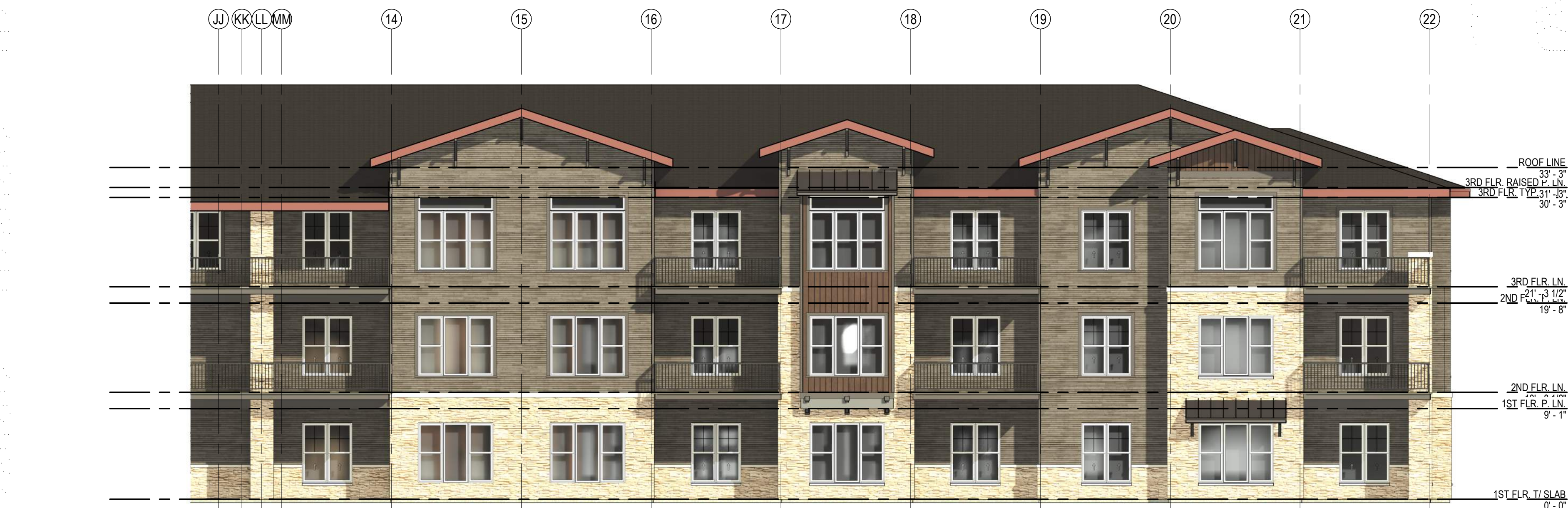
SEGMENT EXTERIOR ELEVATION BLDG. 1 - SEGMENT "A" WEST 1/8" = 1'-0"
