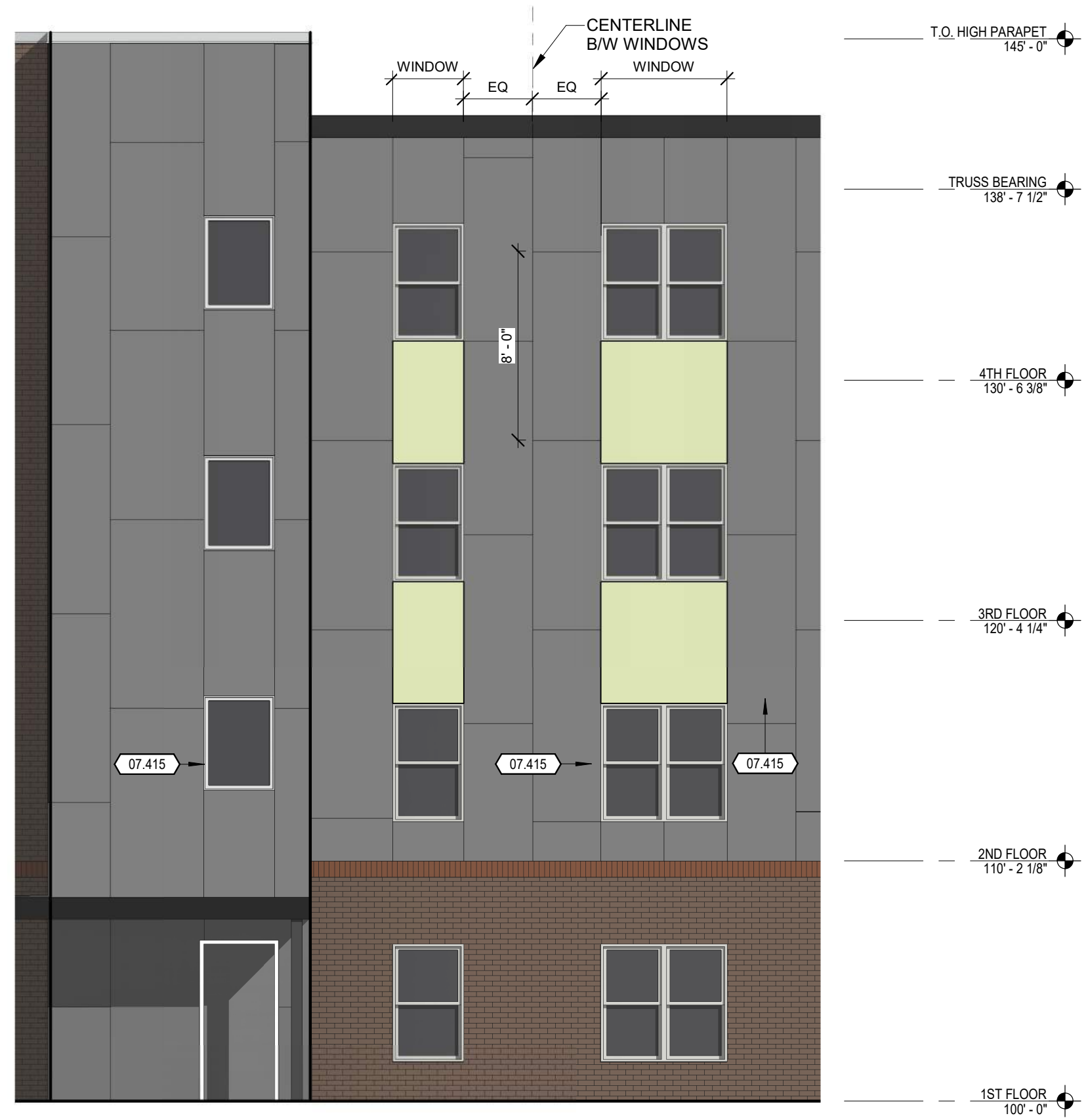
1 EAST ELEVATION - ENLARGED TYPICAL FIBER CEMENT LAYOUT 3/16" = 1'-0"
