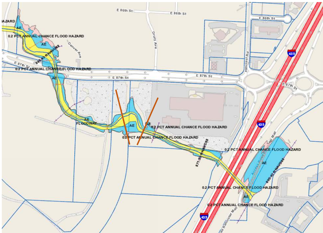
The City's GIS mapping shows the existing FEMA model's floodway and flood hazard zones
