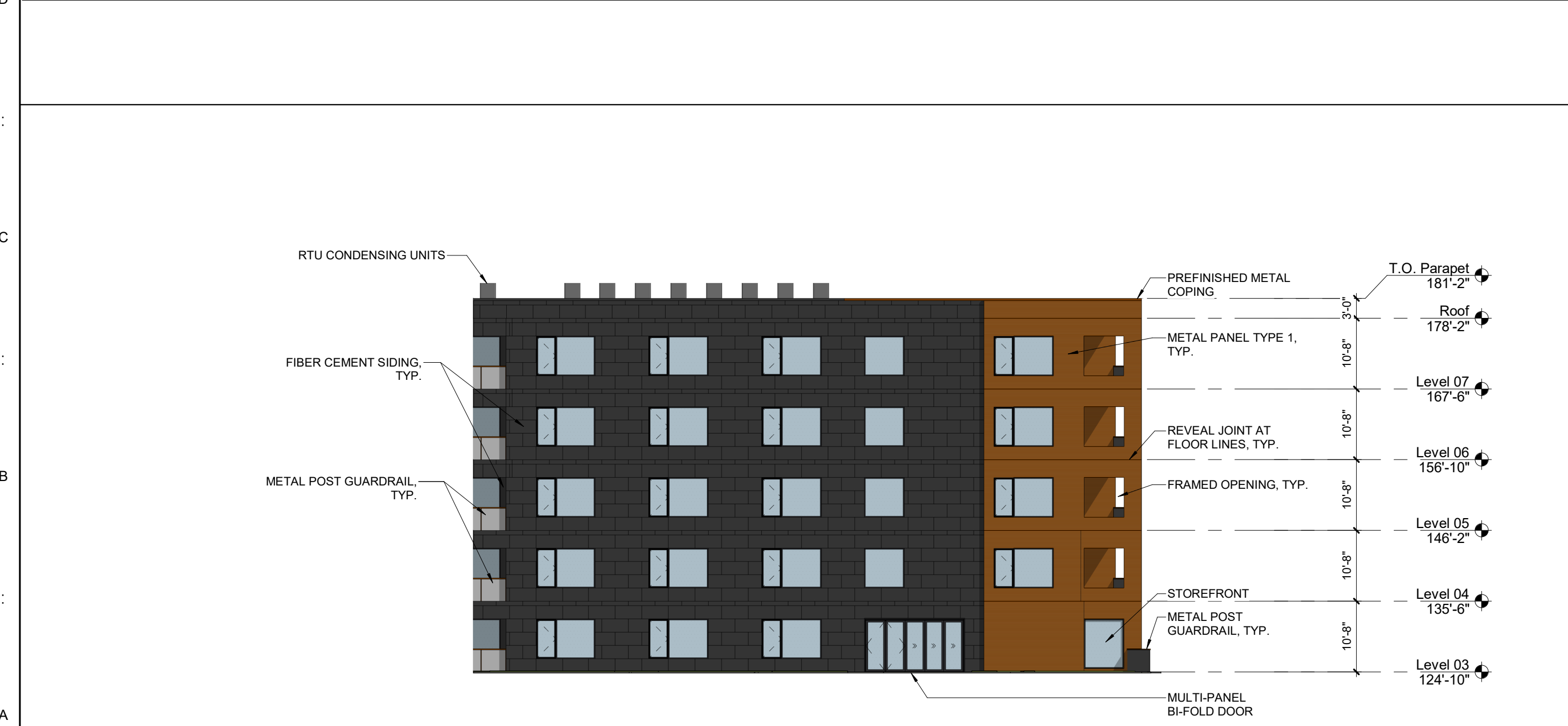
Courtyard - West Elevation A08 1/16" = 1'-0"
