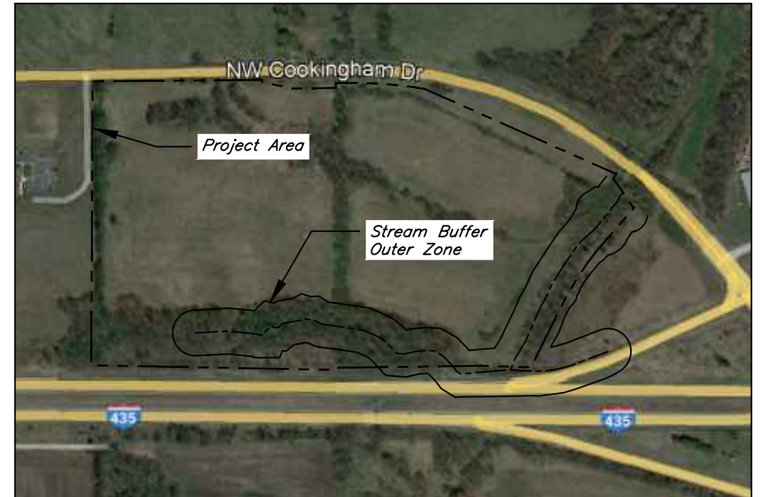
VICINITY MAP Not to Scale KCMO Regulated Stream within Property Boundary: Length = 2426 FT
