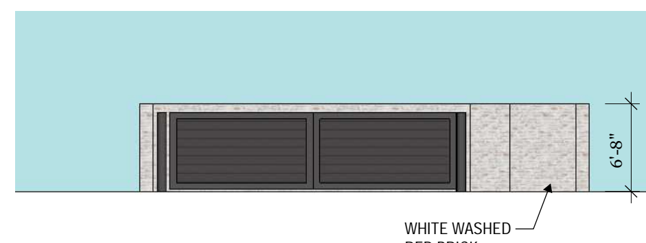
D PRELIMINARY DUMPSTER FRONT SCALE: 1" = 10'
