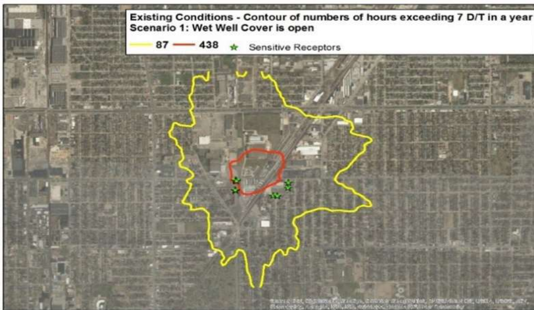
Inside the contours more than the labeled number of hours in a year exceeded the 7 D/T target. Goal for numbers of exceedance: <1% of hours in a year (i.e. < 87 hours per year exceeding 7 D/T)
