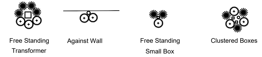
TYPICAL UTILITY BOX SCREENING DETAILS - NTS
