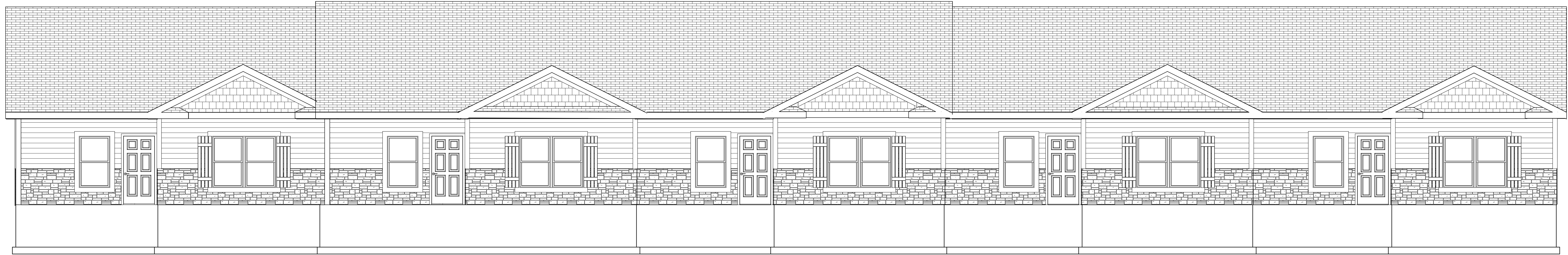
FRONT EL. HARDIE SIDING AND STONE
