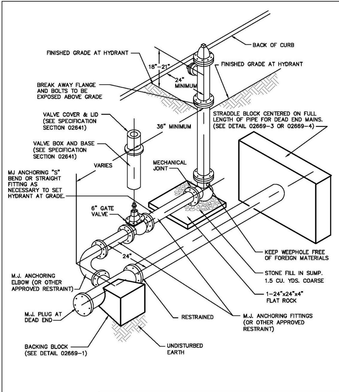
**TYP. HYDRANT INSTALL. WITH 90° BEND
