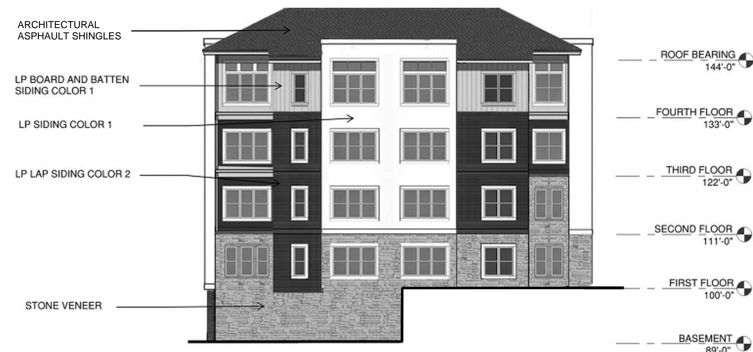
3 BUILDINGS 1, 2 & 4 SIDE ELEVATION 3/32" = 1'-0"
