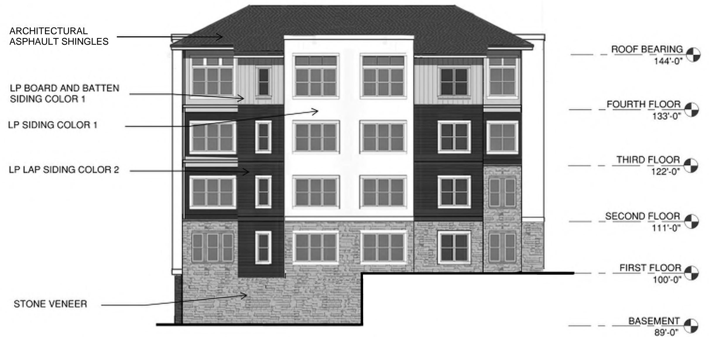
4 BUILDING 3 - SIDE ELEVATION 3/32" = 1'-0"
