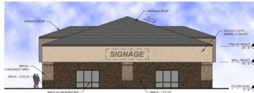
EXTERIOR ELEVATION - SOUTH SCALE: 1/8" = 1'-0"
