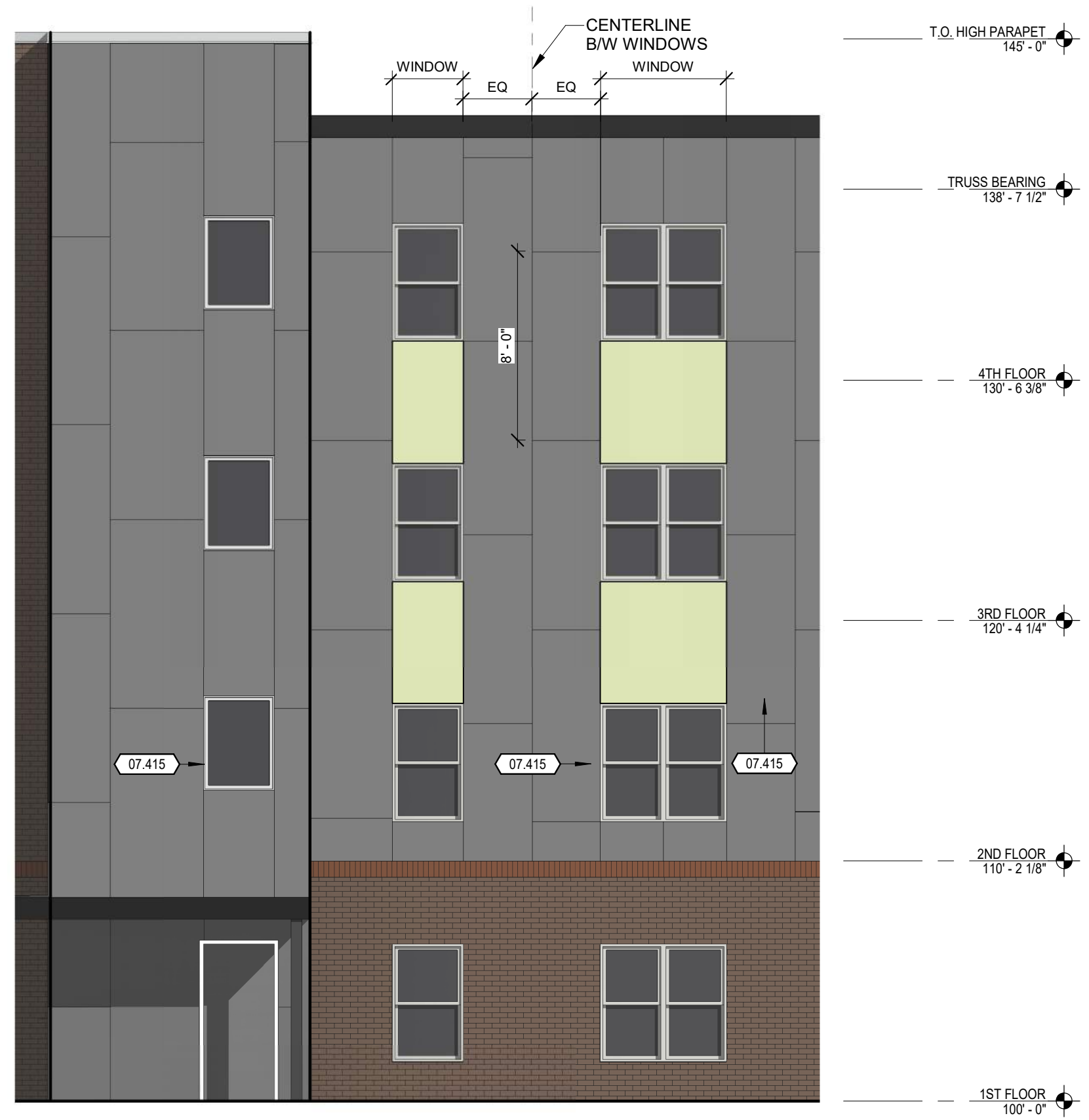
1 EAST ELEVATION - ENLARGED TYPICAL FIBER CEMENT LAYOUT 3/16" = 1'-0"
