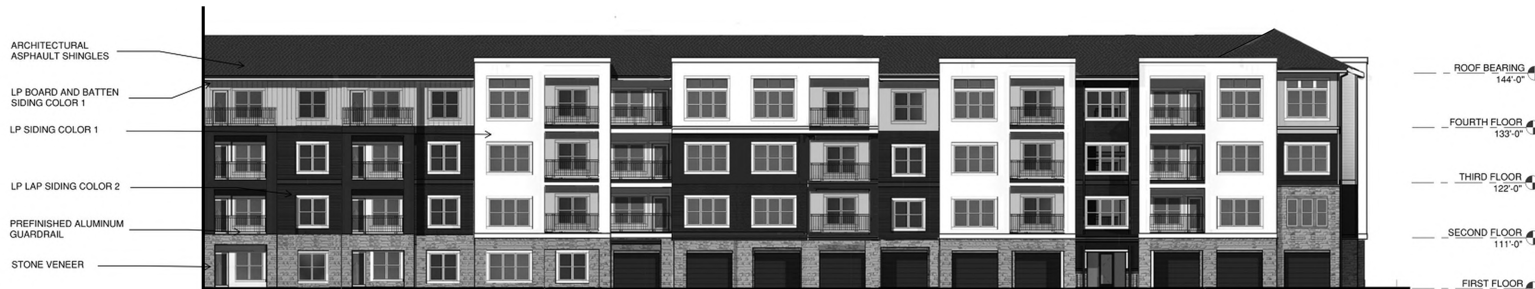
1 BUILDING 1 - FRONT ELEVATION 3/32" = 1'-0"
