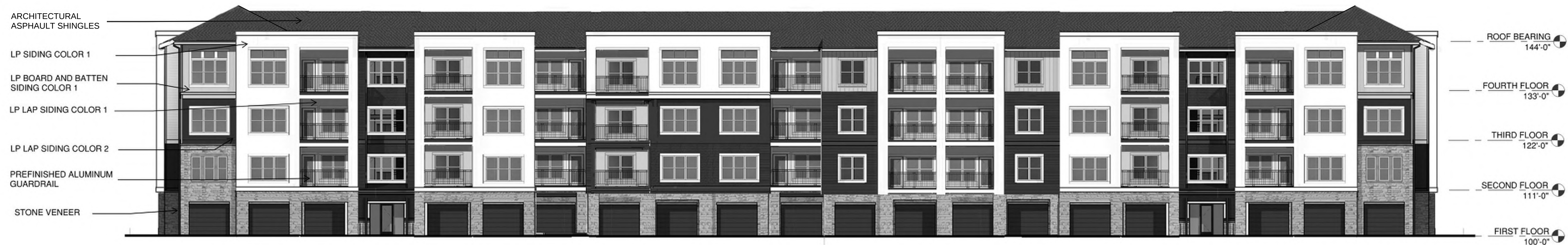
2 BUILDINGS 2 & 4 - FRONT ELEVATION 3/32" = 1'-0"
