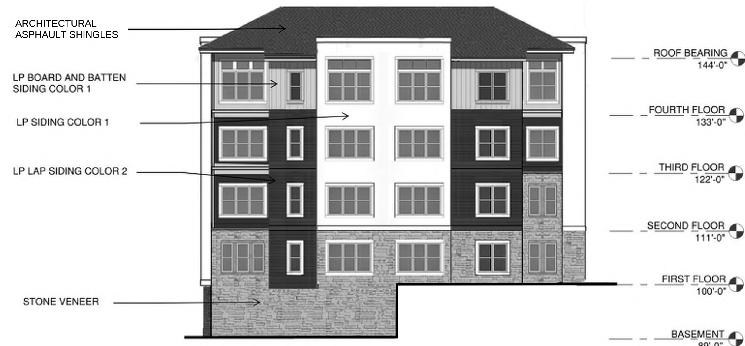
3 BUILDINGS 1, 2 & 4 SIDE ELEVATION 3/32" = 1'-0"
