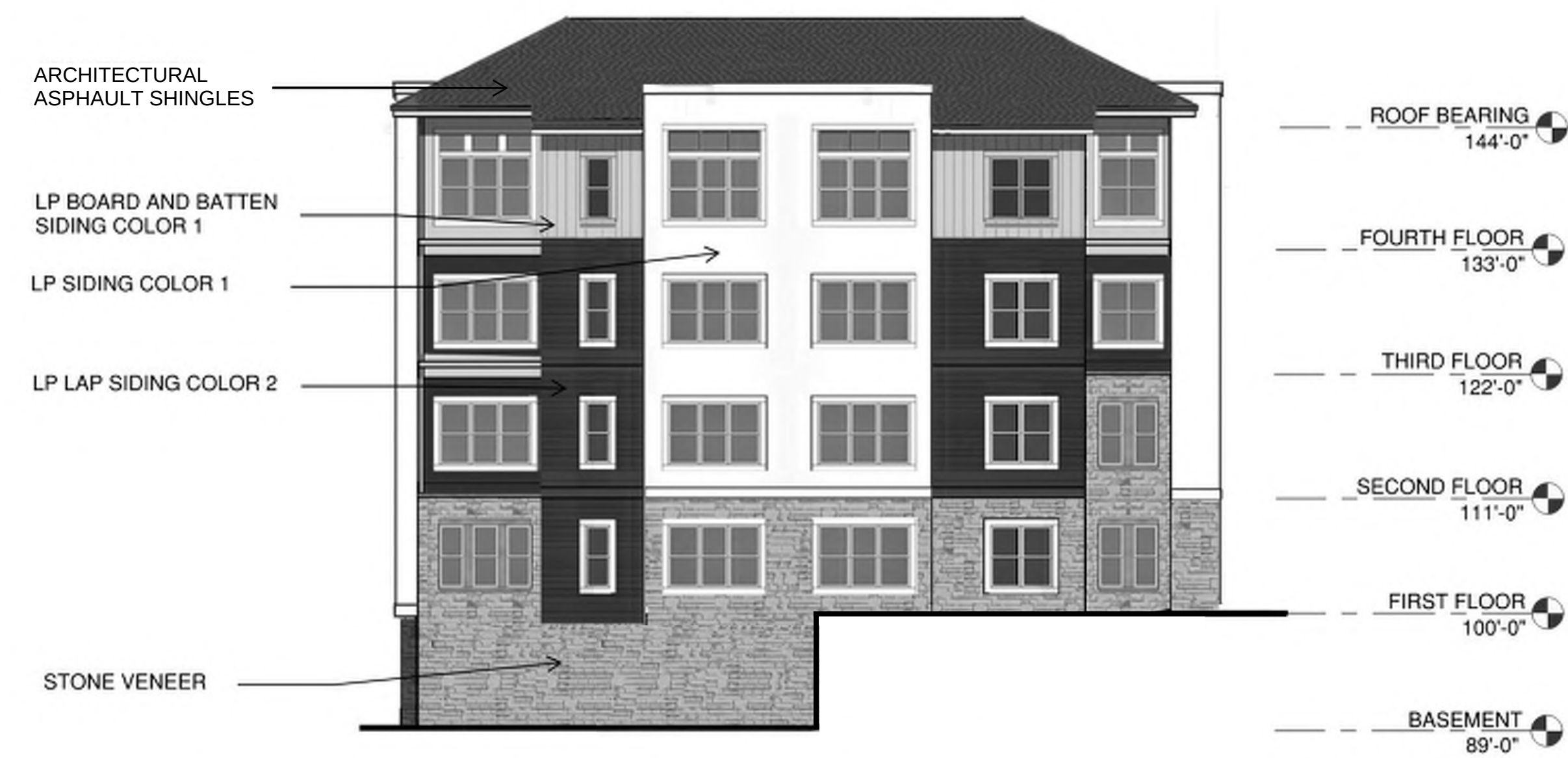
4 BUILDING 3 - SIDE ELEVATION 3/32" = 1'-0"
