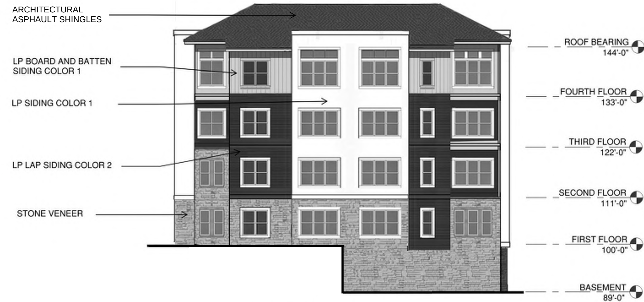
4 BUILDINGS 1, 2 & 4 SIDE ELEVATION 3/32" = 1'-0"
