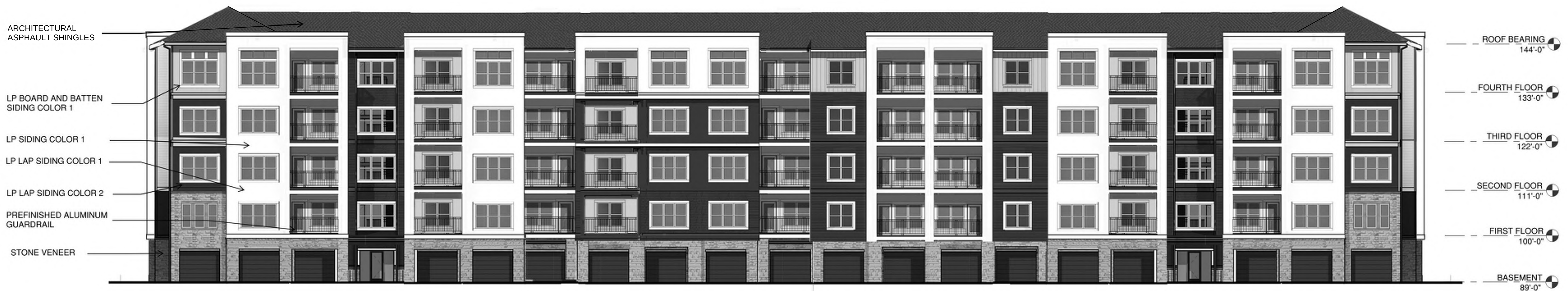
2 BUILDING 3 - FRONT ELEVATION 3/32" = 1'-0"
