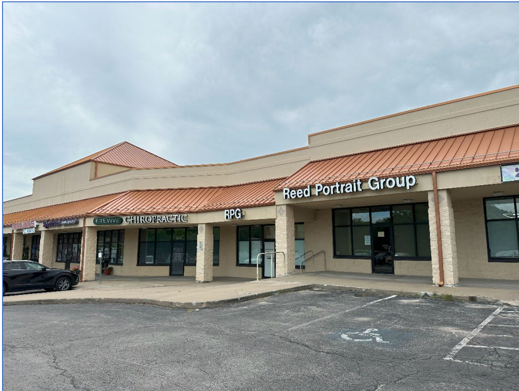
Looking east – cracked/uneven pavement (fall/trip hazard); lack of ADA signage; drainage across sidewalk
