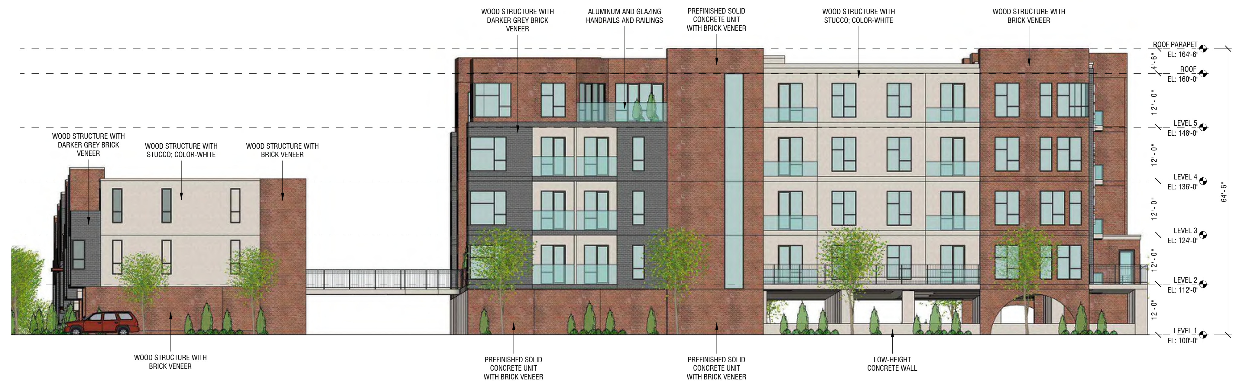
2 SOUTH ELEVATION - W 34TH TERRACE 1/2" = 1'-0"
