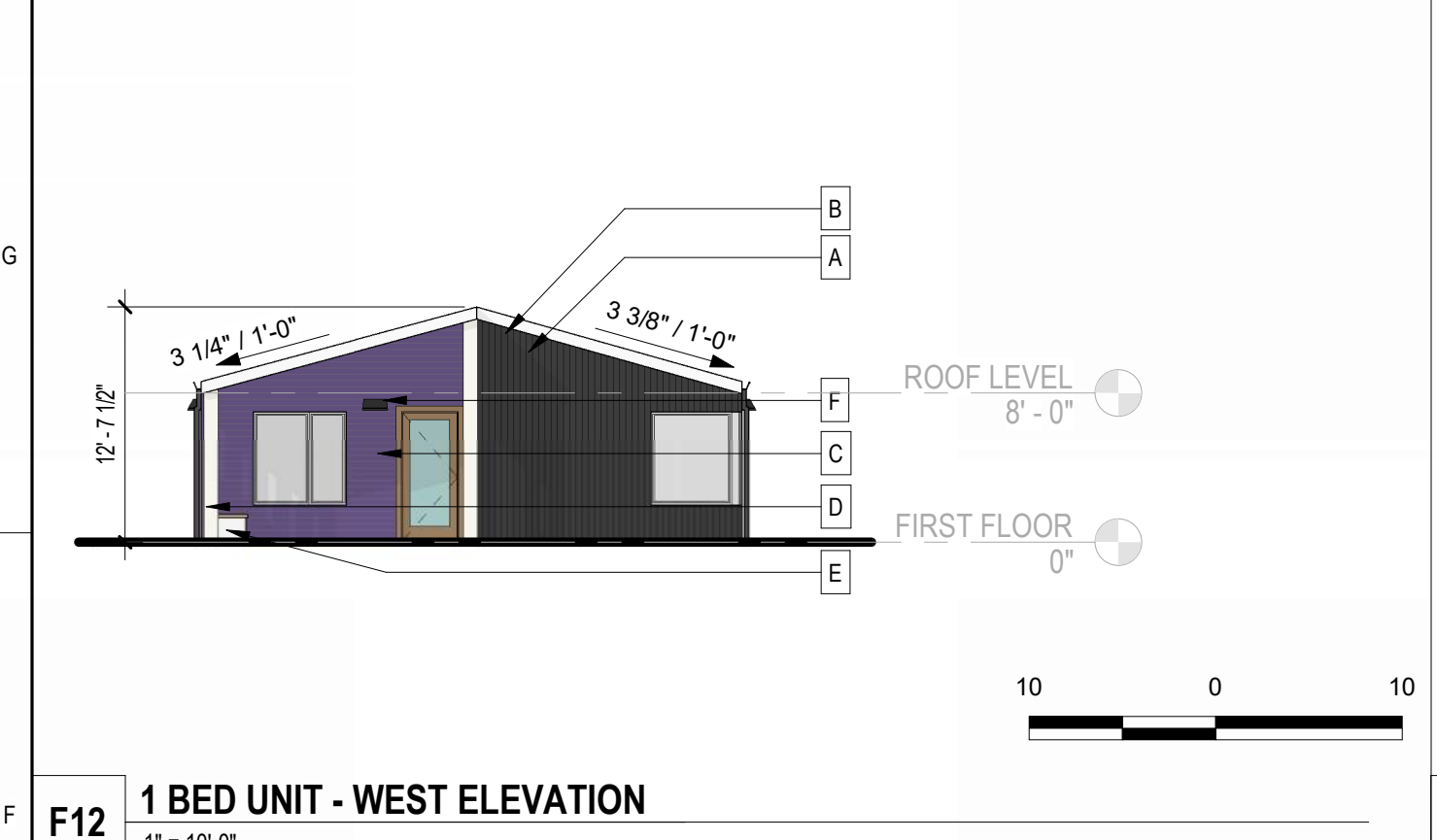
F12 1 BED UNIT - WEST ELEVATION 1" = 10'-0"
