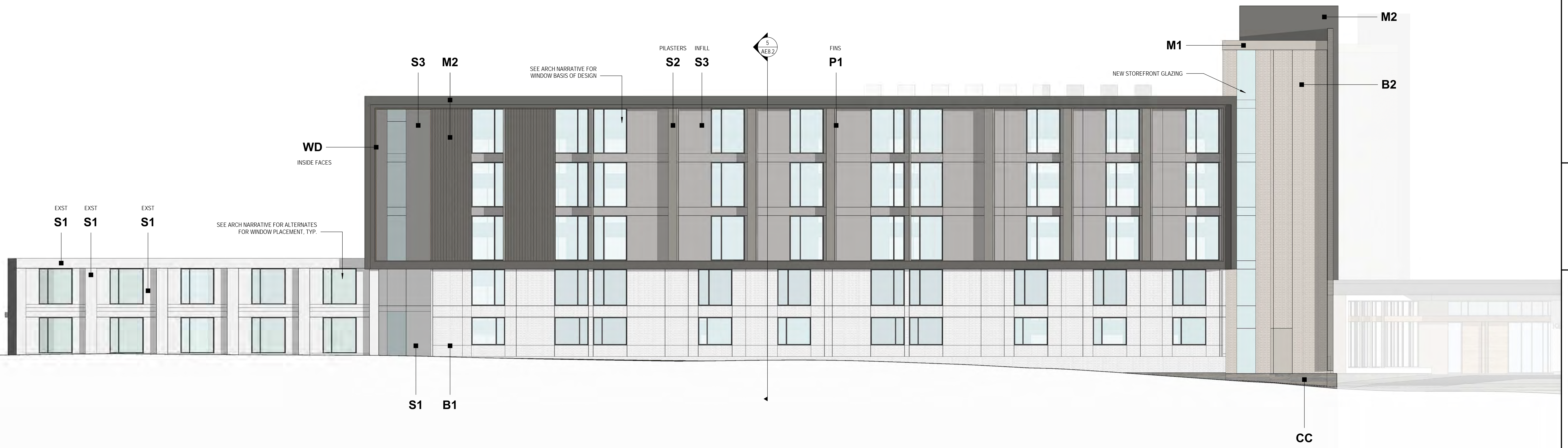
NORTH ELEVATION / NEW GUESTROOM TOWER
