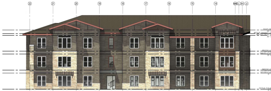
2 SEGMENT EXTERIOR ELEVATION BLDG. 1 - SEGMENT "A" EAST 1/8" = 1'-0"
