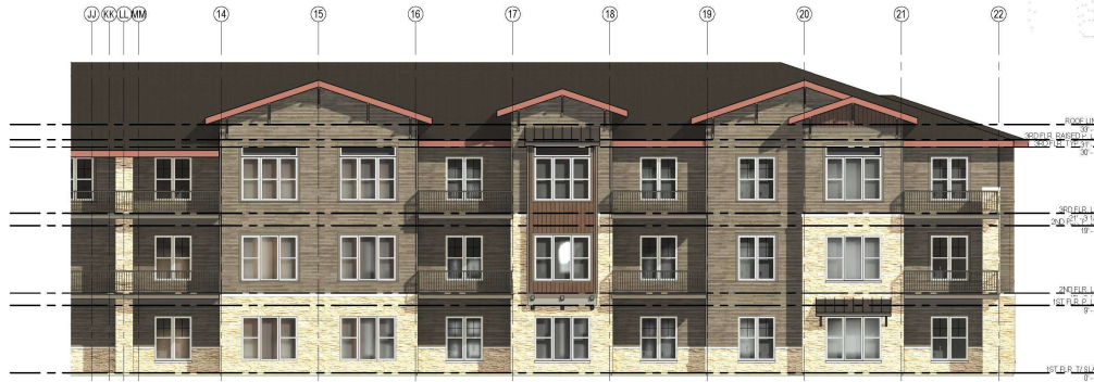
1 SEGMENT EXTERIOR ELEVATION BLDG. 1 - SEGMENT "A" WEST 1/8" = 1'-0"
