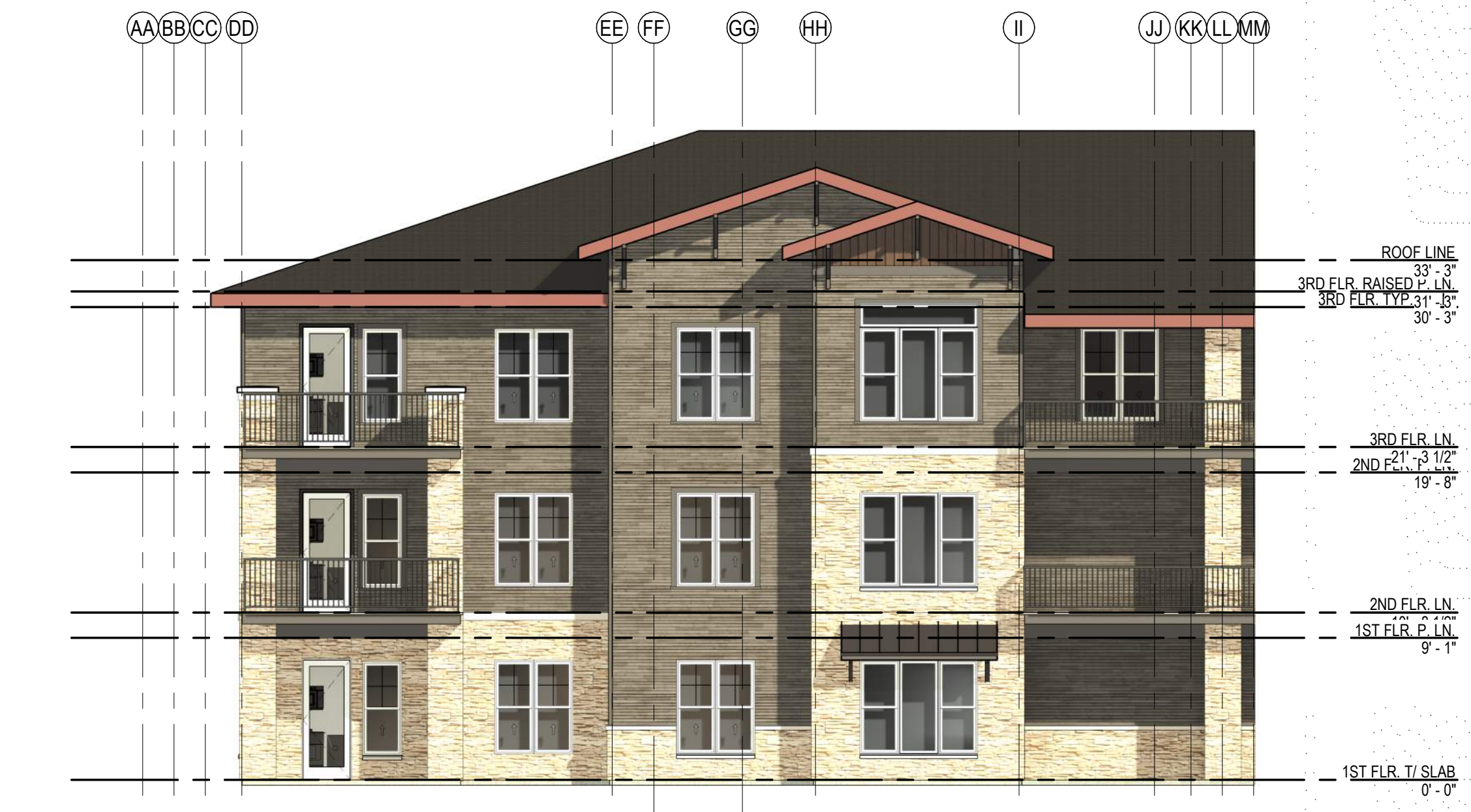
2 SEGMENT EXTERIOR ELEVATION BLDG. 1 - SEGMENT "B" WEST 1/8" = 1'-0"
