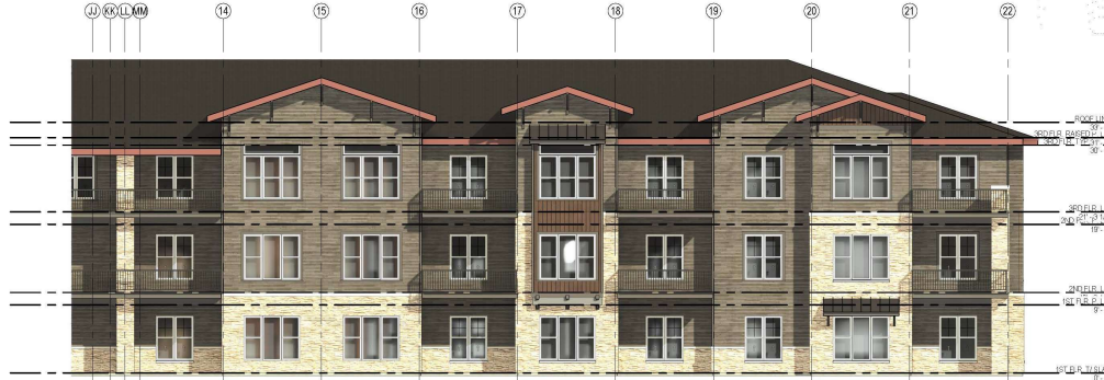
1 SEGMENT EXTERIOR ELEVATION BLDG. 1 - SEGMENT "A" WEST 1/8" = 1'-0"
