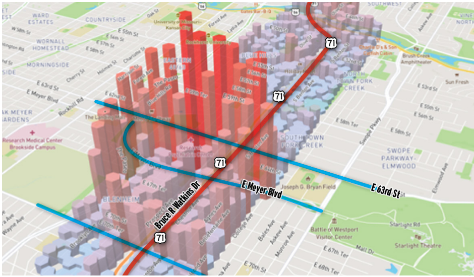
Our data-driven approach will utilize existing innovative data sources such as StreetLight to understand pedestrian activity using 3D heat maps of the US-71 corridor as shown above.
