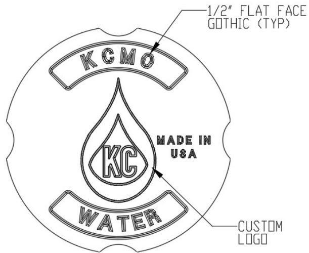
**Figure 3: Standard Valve Cover Markings**
