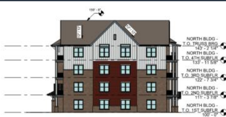
3 NORTH BUILDING - EAST ELEVATION 1/16" = 1'-0"
