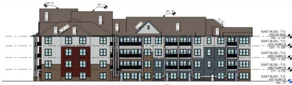
4 EAST BUILDING - WEST ELEVATION 1/16" = 1'-0"
