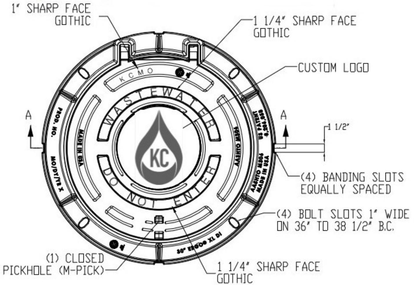
**Figure 1: Standard Sanitary Sewer Manhole Markings For Ductile Iron Castings**
