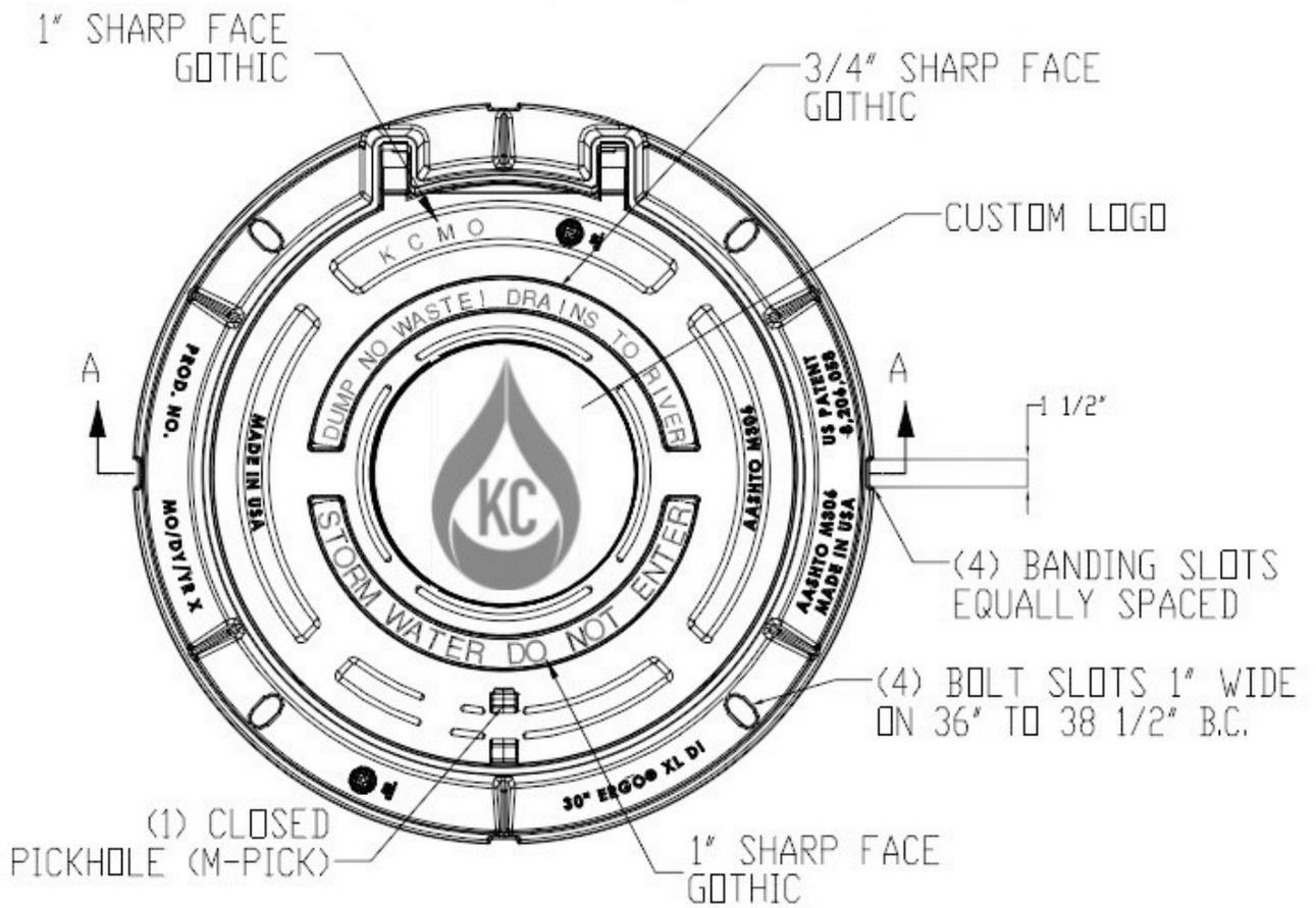
**Figure 1: Standard Stormwater Markings**
