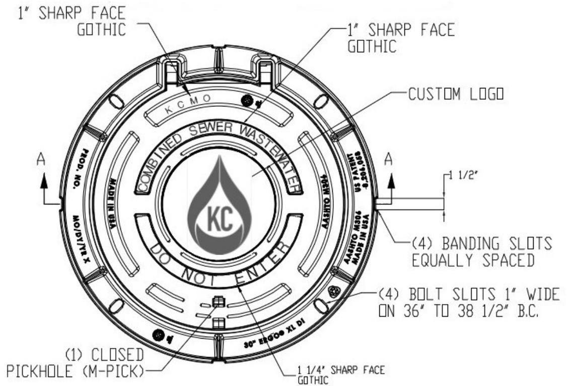
**Figure 2: Optional Sanitary Sewer Manhole Markings
