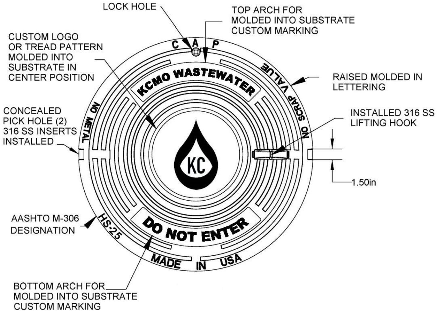
**Figure 3: Standard Sanitary Sewer Manhole Markings For Composite Castings**
