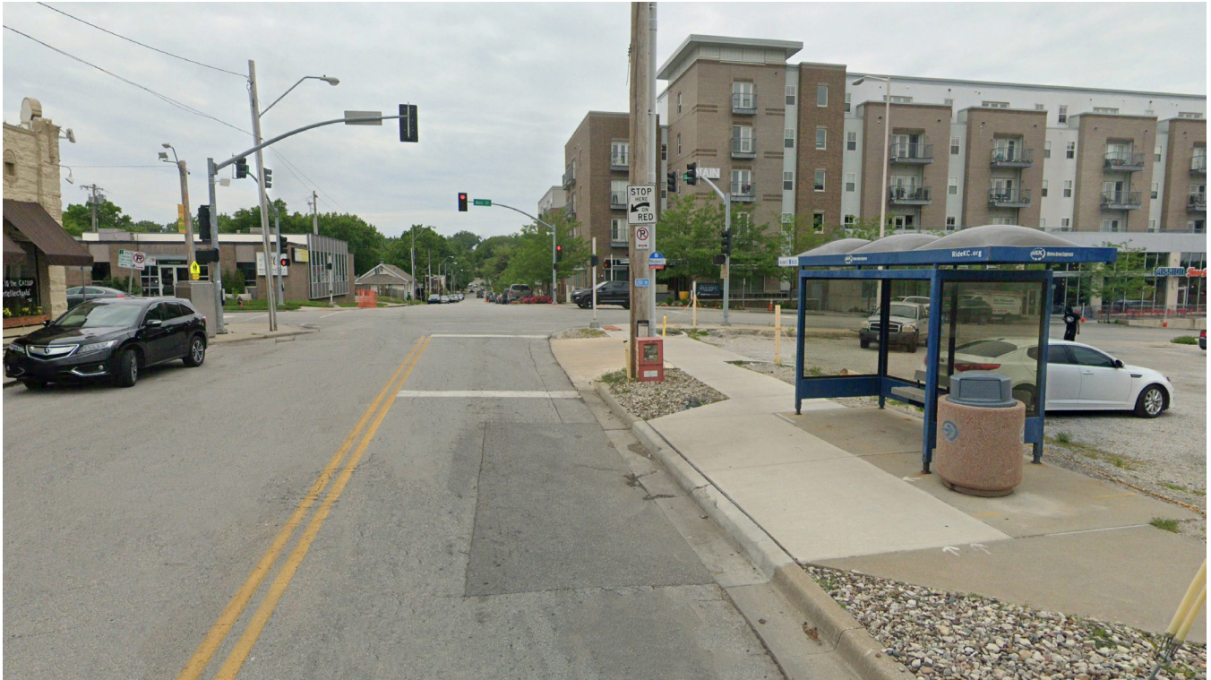
Figure 5 – Recessed stop bar
