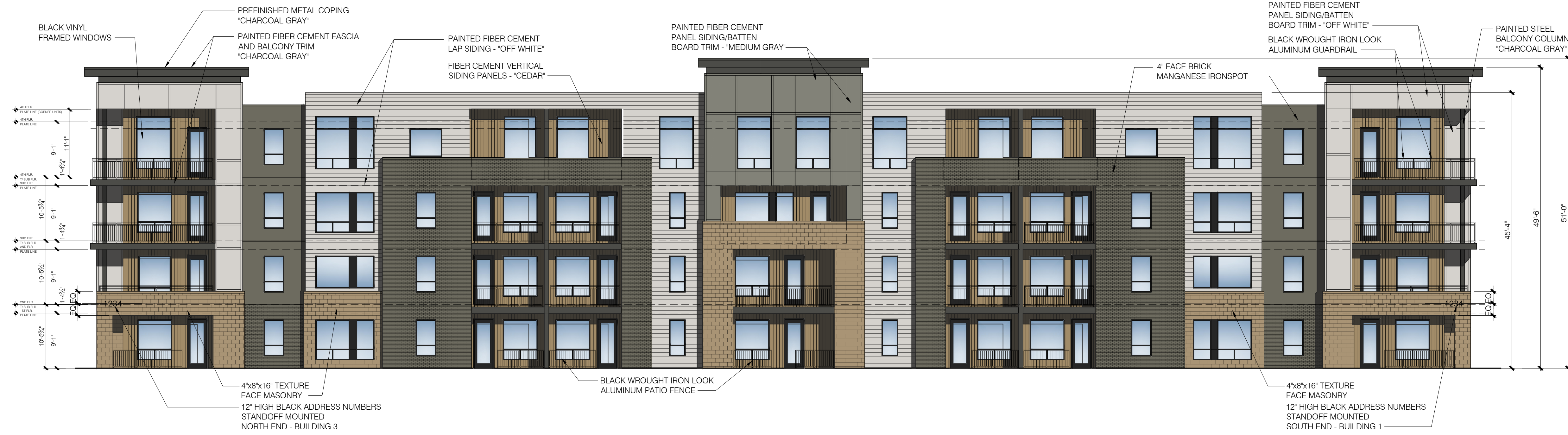
2 BUILDING 1&3 WEST ELEVATION
