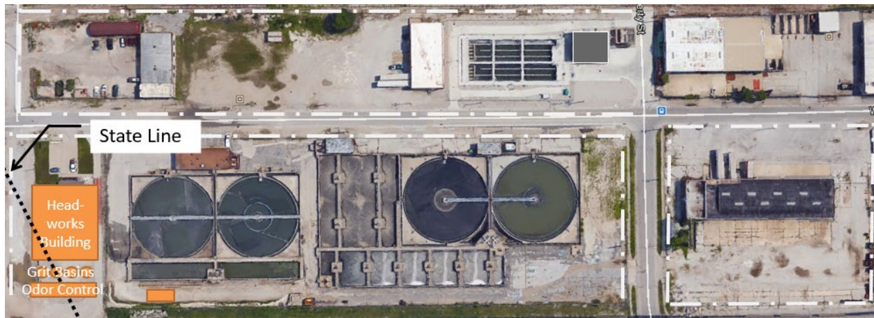
Figure 1: Westside Treatment Plant Headworks (Aerial Plan)
