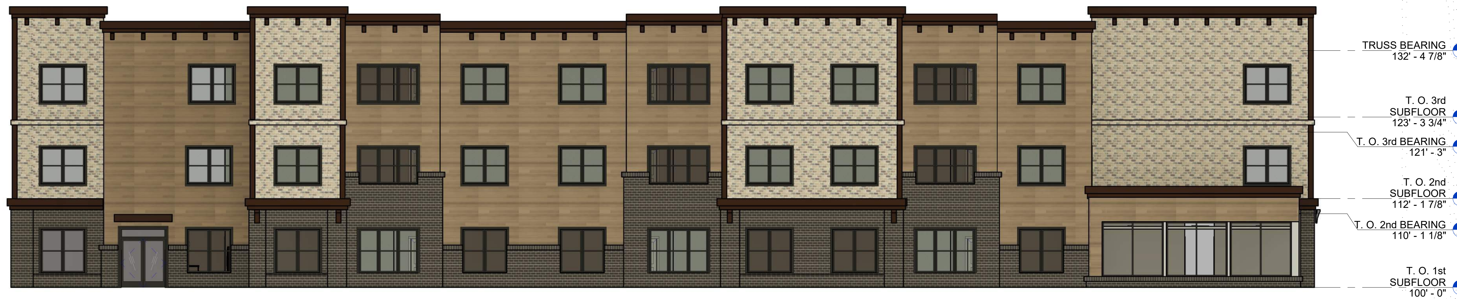
A1 APARTMENTS - EAST ELEVATION (TRACY AVE) 1/8" = 1'-0"
