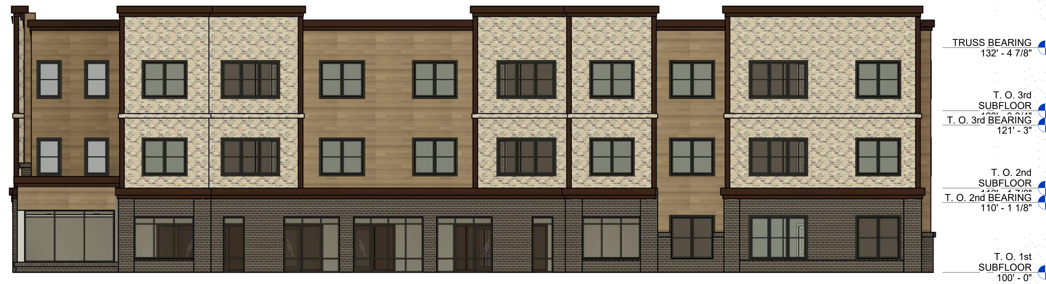
B1 APARTMENTS - NORTH ELEVATION 1/8" = 1'-0"
