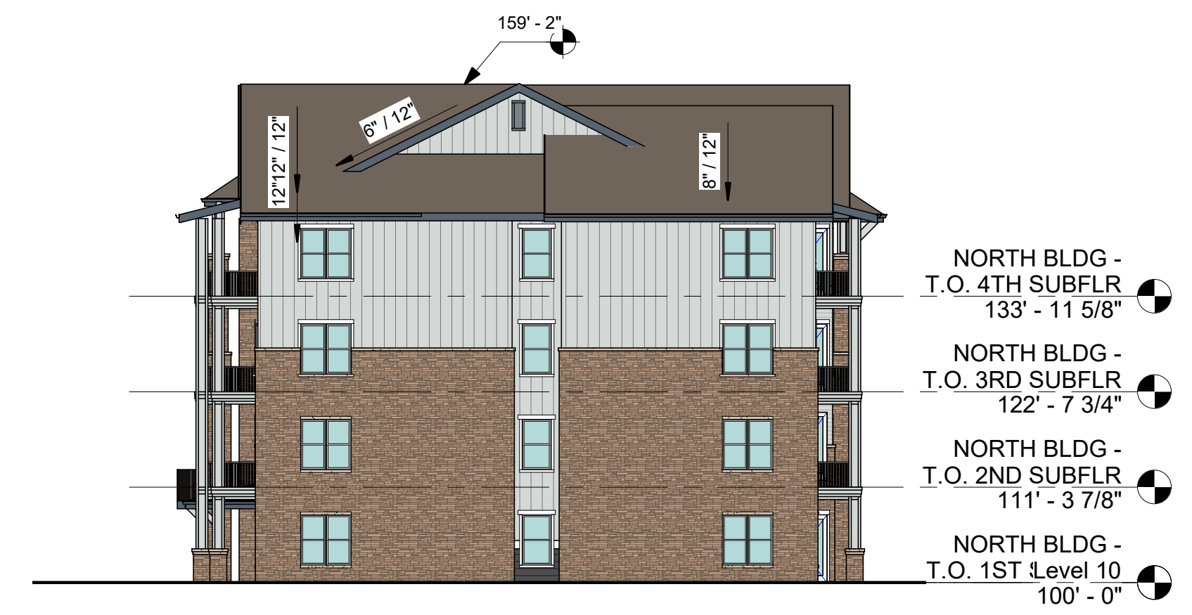
4 NORTH BUILDING - WEST ELEVATION 1/16" = 1'-0"
