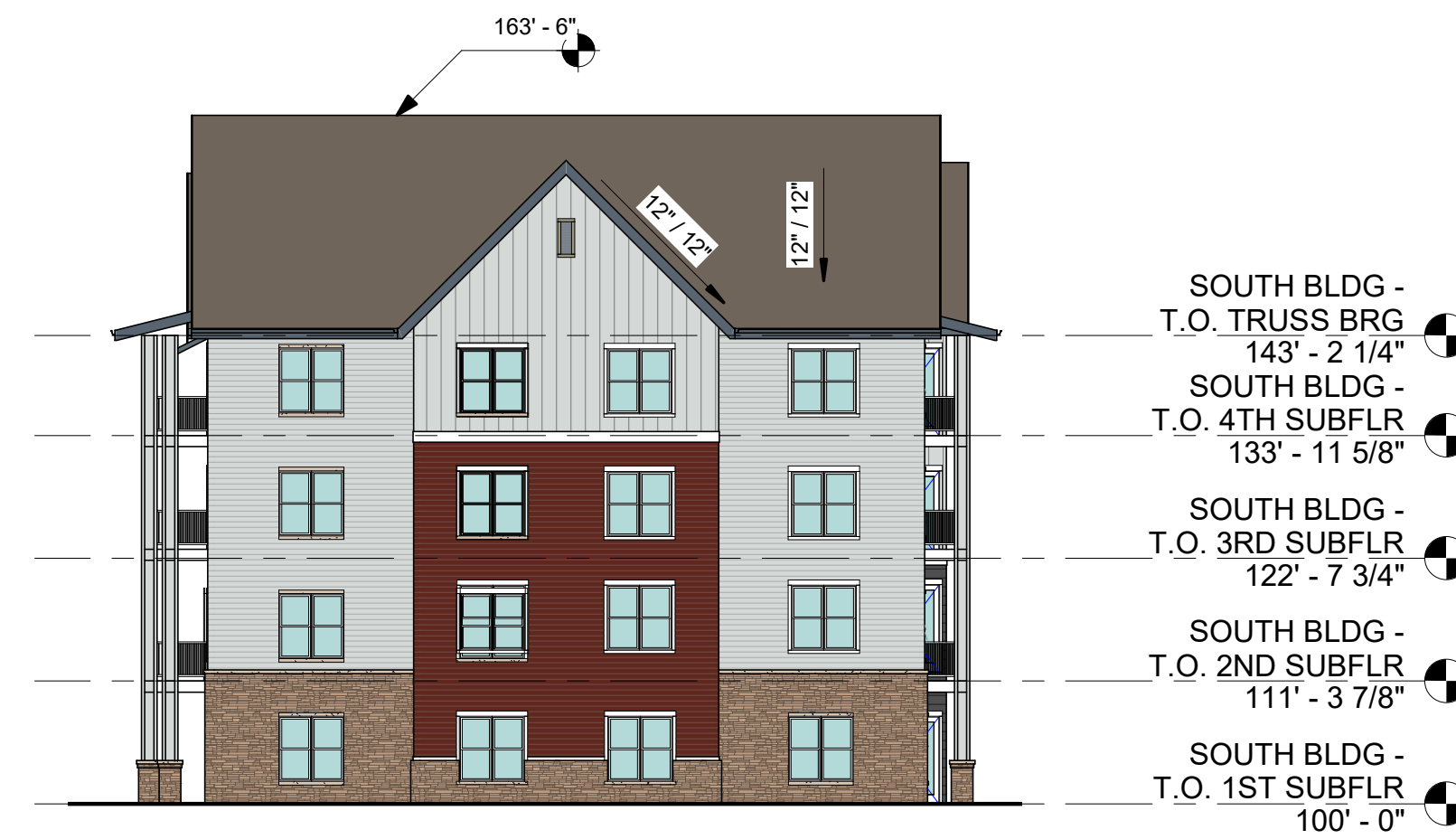
4 SOUTH BUILDING - WEST ELEVATION 1/16" = 1'-0"
