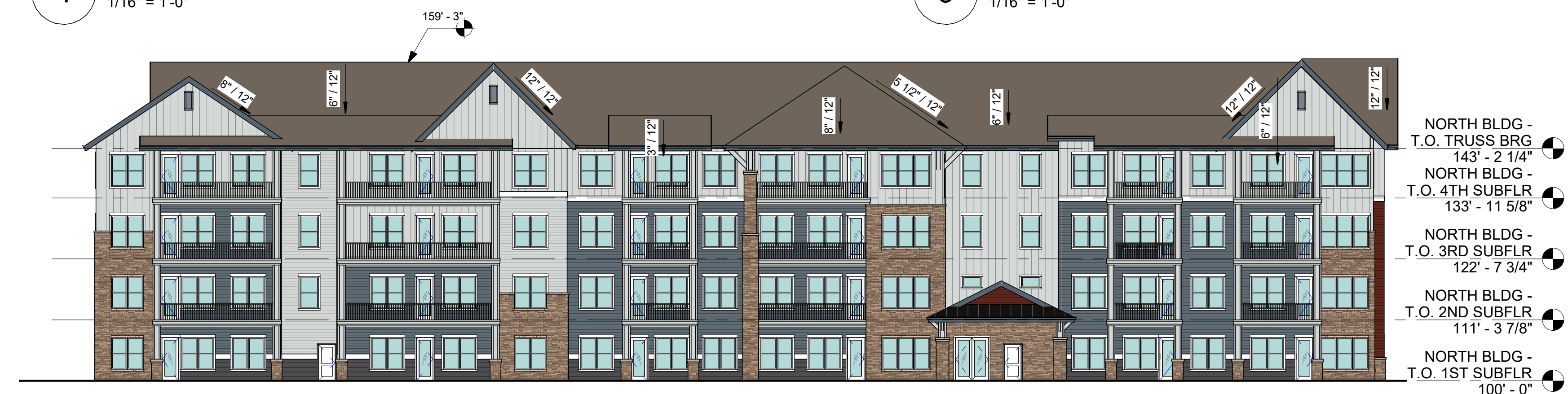
2 NORTH BUILDING - SOUTH ELEVATION 1/16" = 1'-0"
