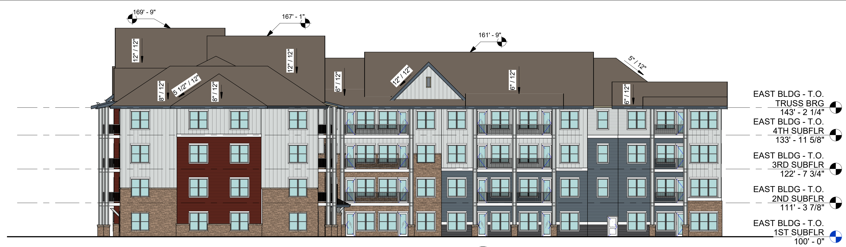
4 EAST BUILDING - WEST ELEVATION 1/16" = 1'-0"
