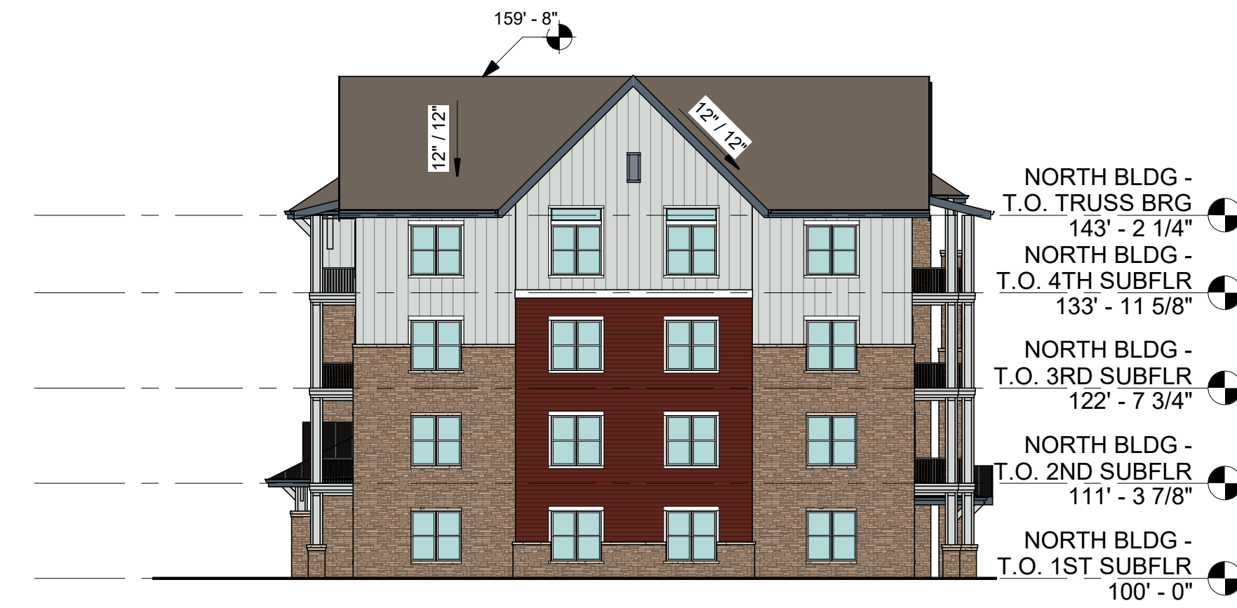
3 NORTH BUILDING - EAST ELEVATION 1/16" = 1'-0"
