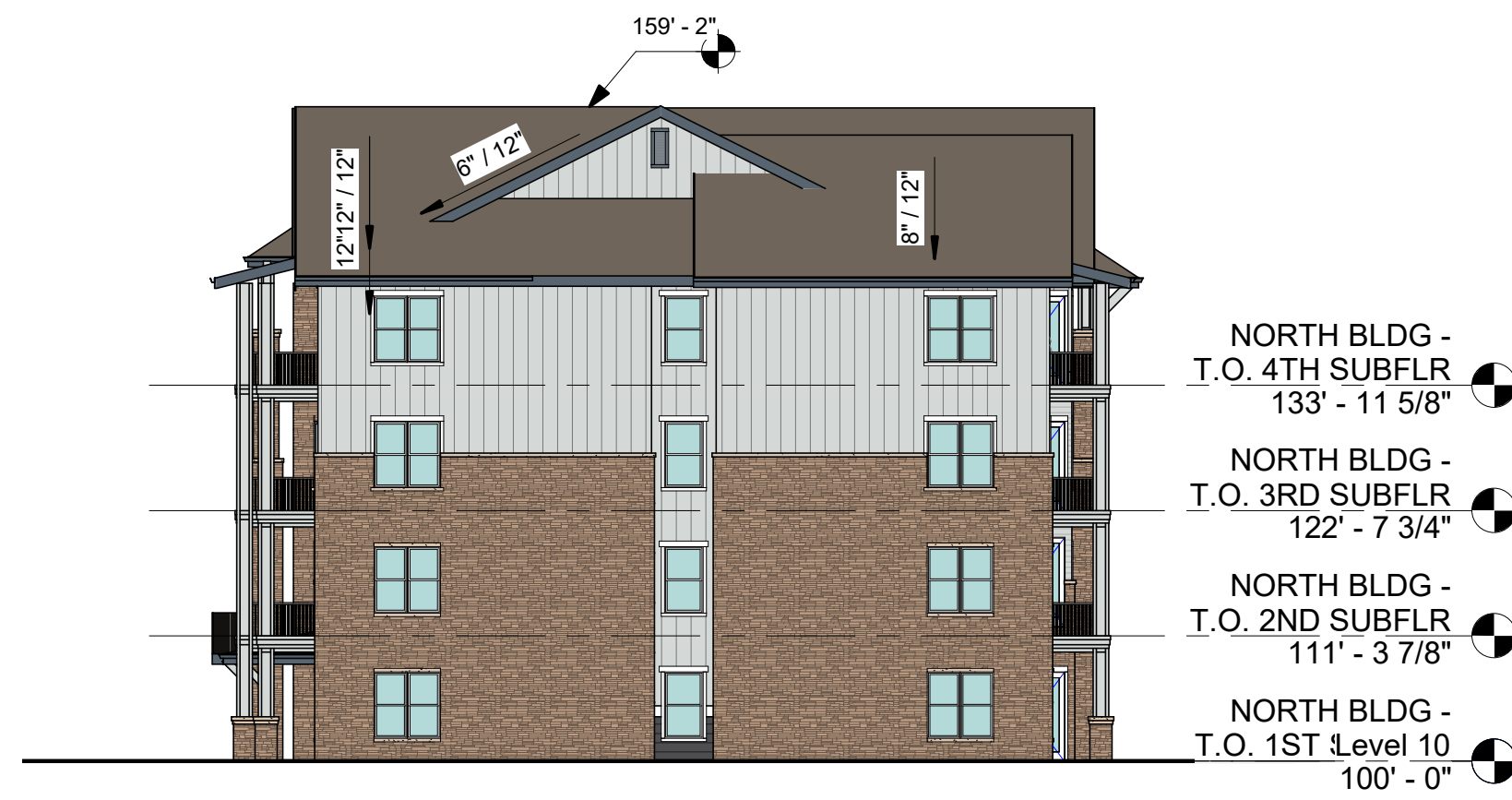
4 NORTH BUILDING - WEST ELEVATION 1/16" = 1'-0"
