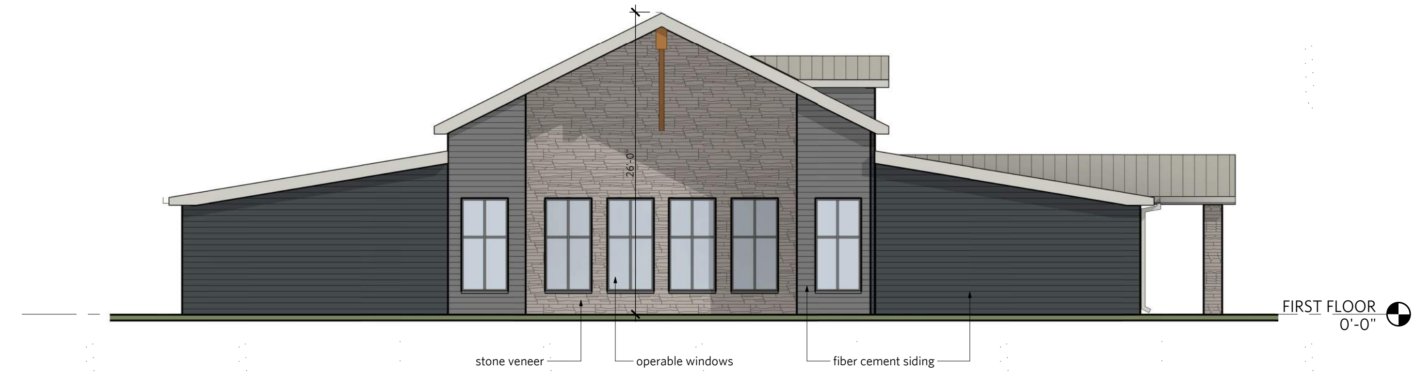
3 | Elevation - HALO Housing - West 1/8" = 1'-0"
