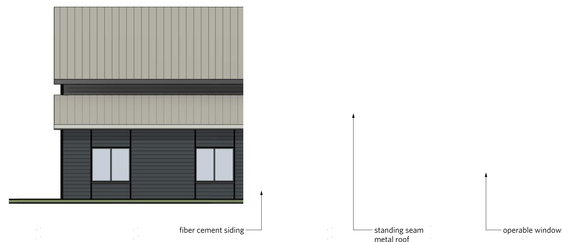
2 | Elevation - HALO Housing - North 1/8" = 1'-0"
