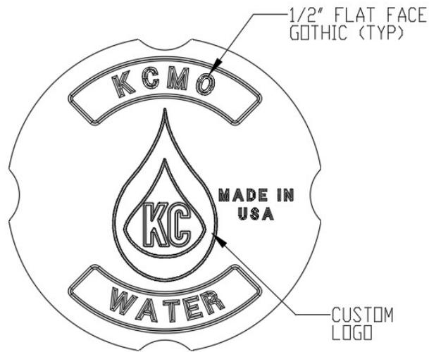
**Figure 3: Standard Valve Cover Markings**
