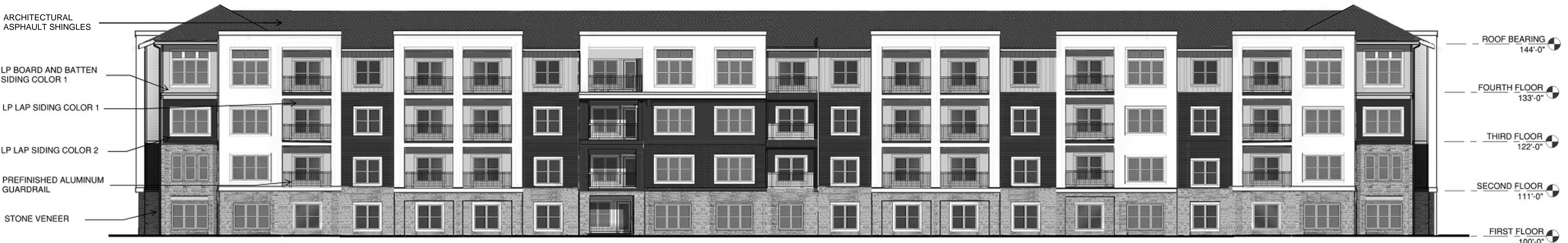
1 BUILDING 3 - REAR ELEVATION 3/32" = 1'-0"
