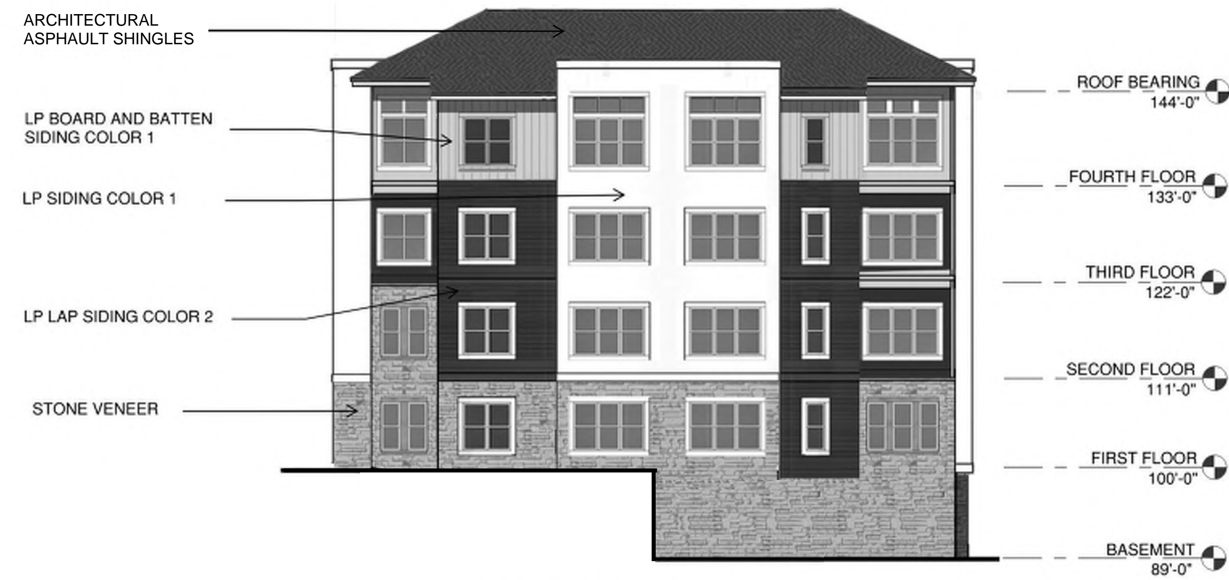
4 BUILDINGS 1, 2 & 4 SIDE ELEVATION 3/32" = 1'-0"
