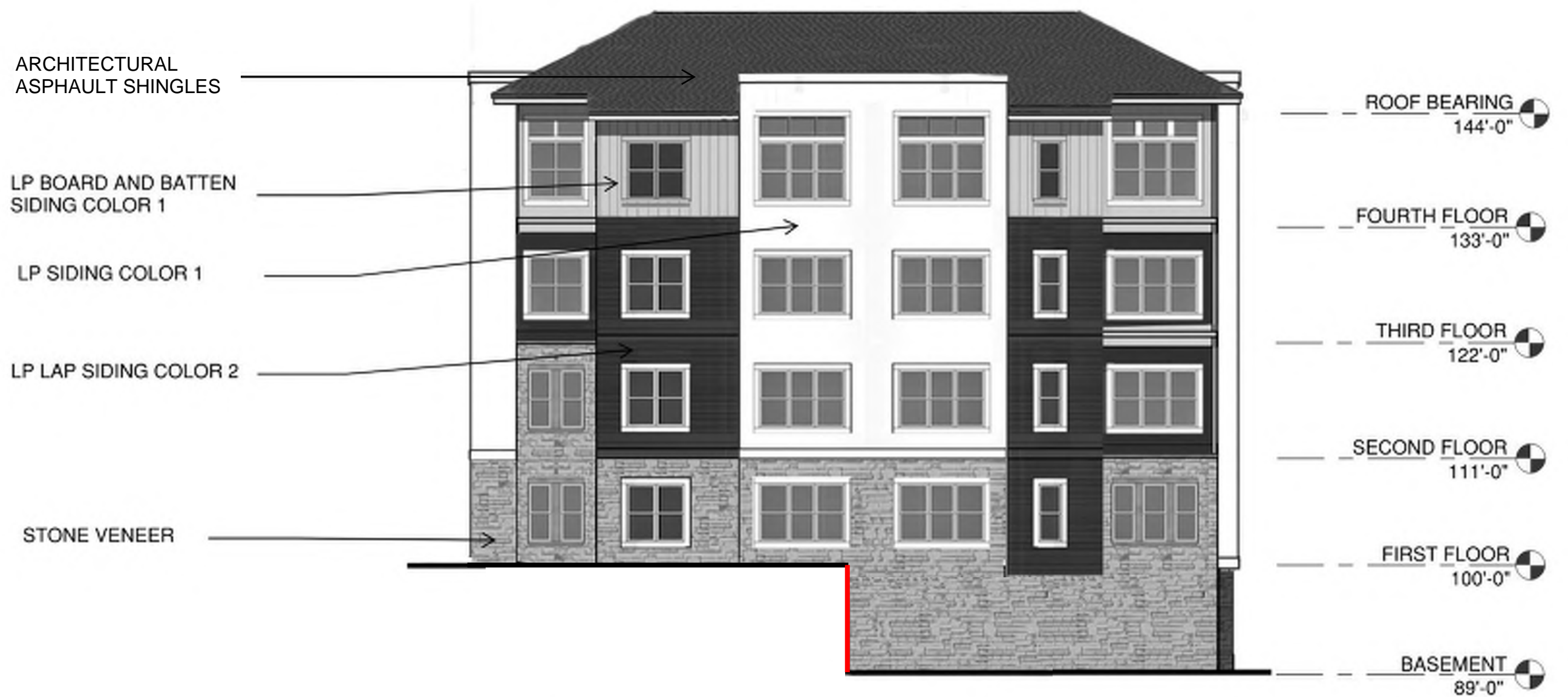
3 BUILDING 3 - SIDE ELEVATION 3/32" = 1'-0"
