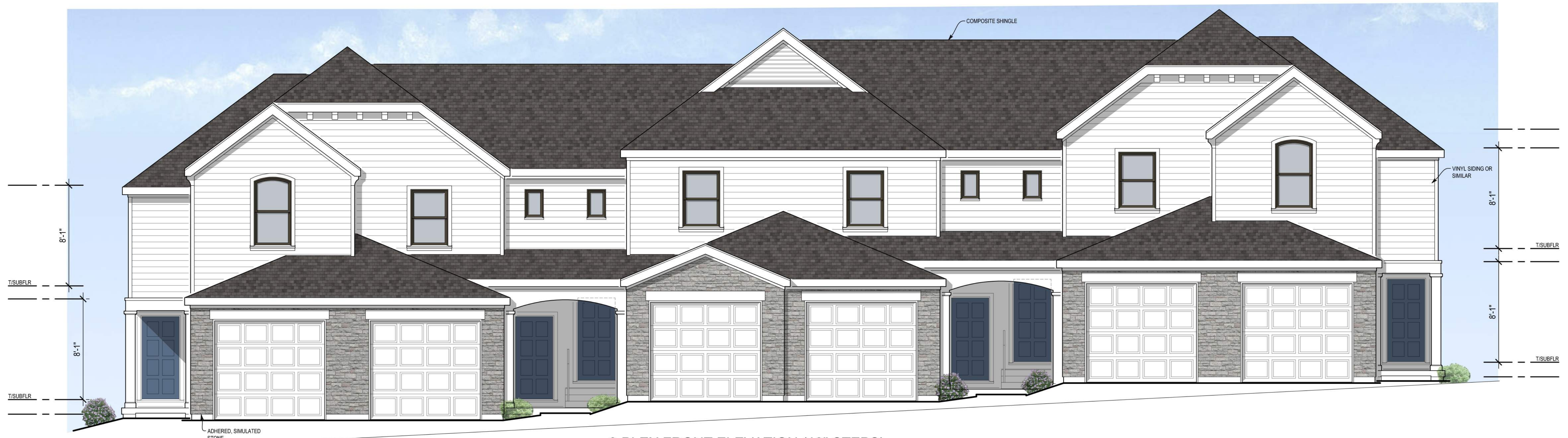
6-PLEX FRONT ELEVATION (18" STEPS) 1/4" = 1'-0"
