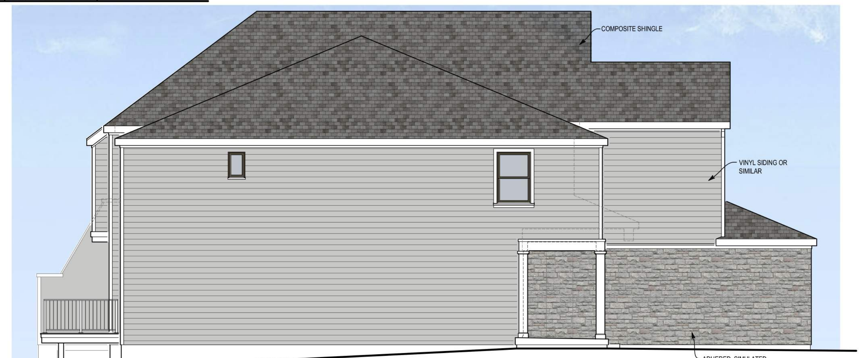
4-PLEX LEFT ELEVATION 3/16" = 1'-0"
