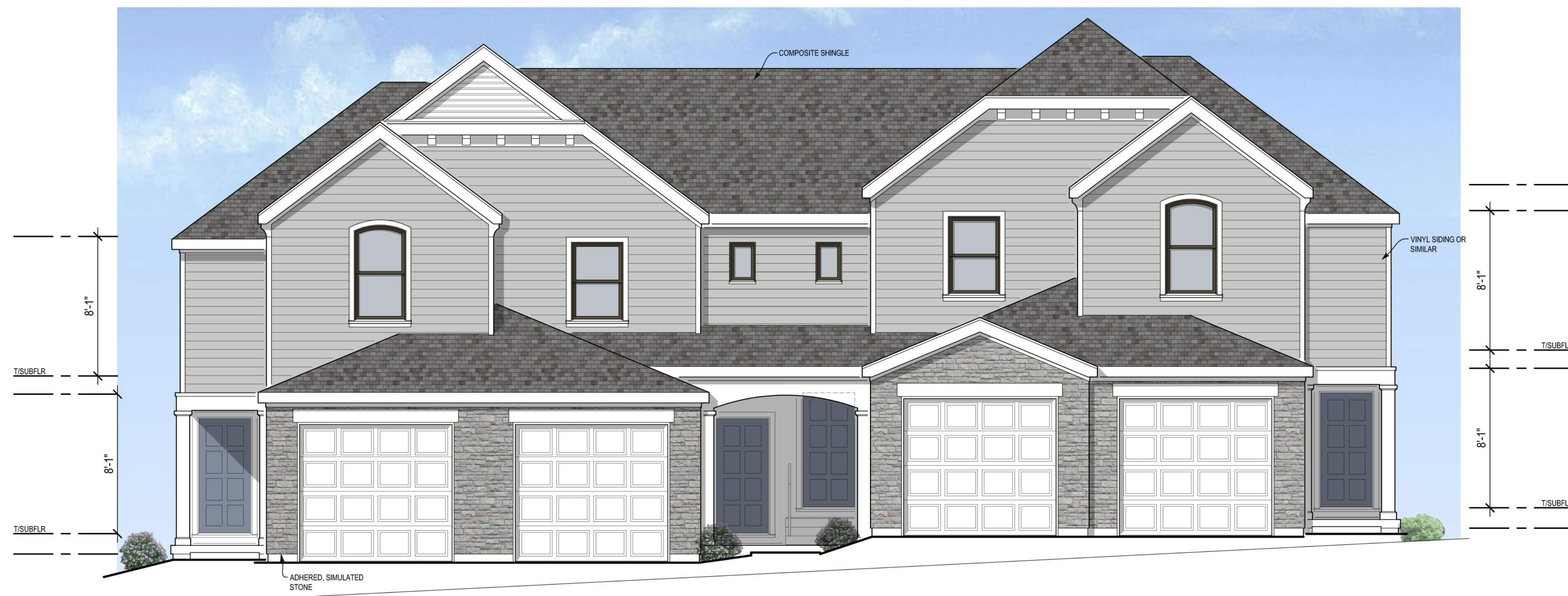
4-PLEX FRONT ELEVATION (18" STEPS) 1/4" = 1'-0"
