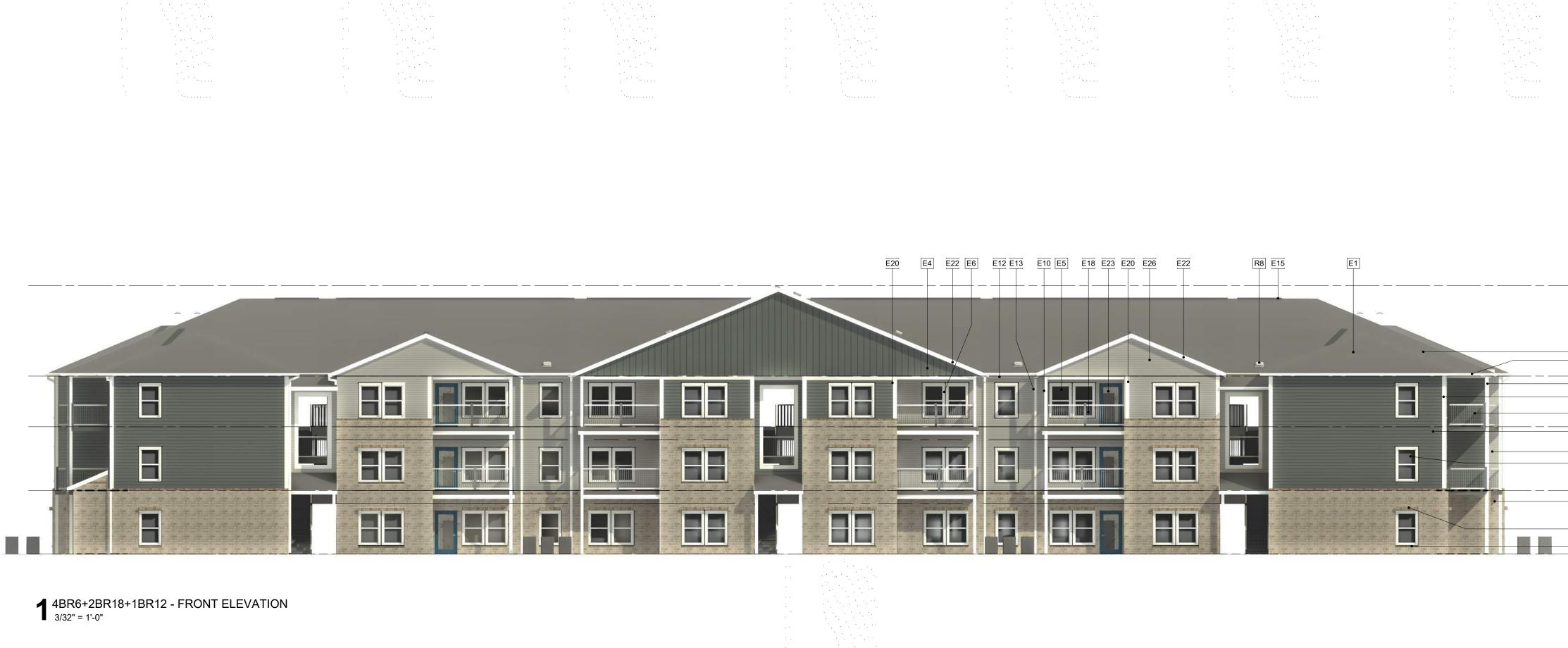
42'-5" HIGH ROOF RIDGE - 28'-1 1/4" ROOF BEARING POINT Н 20'-1 1/4" THIRD FLOOR EE 88 10'-0 5/8" SECOND FLOOR P FNTE 0" FIRST FLOOR
