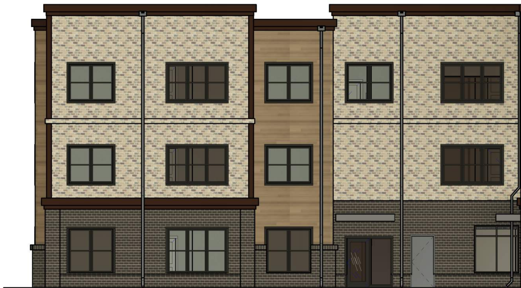
B2 APARTMENTS - SOUTH ELEVATION 1/8" = 1'-0"
