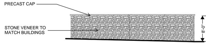
**7 TRASH ENCLOSURE - WEST ELEVATION**
