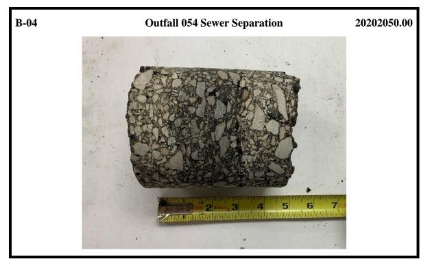
MaterialThickness (in)Asphalt4.75Base gravel0.75
