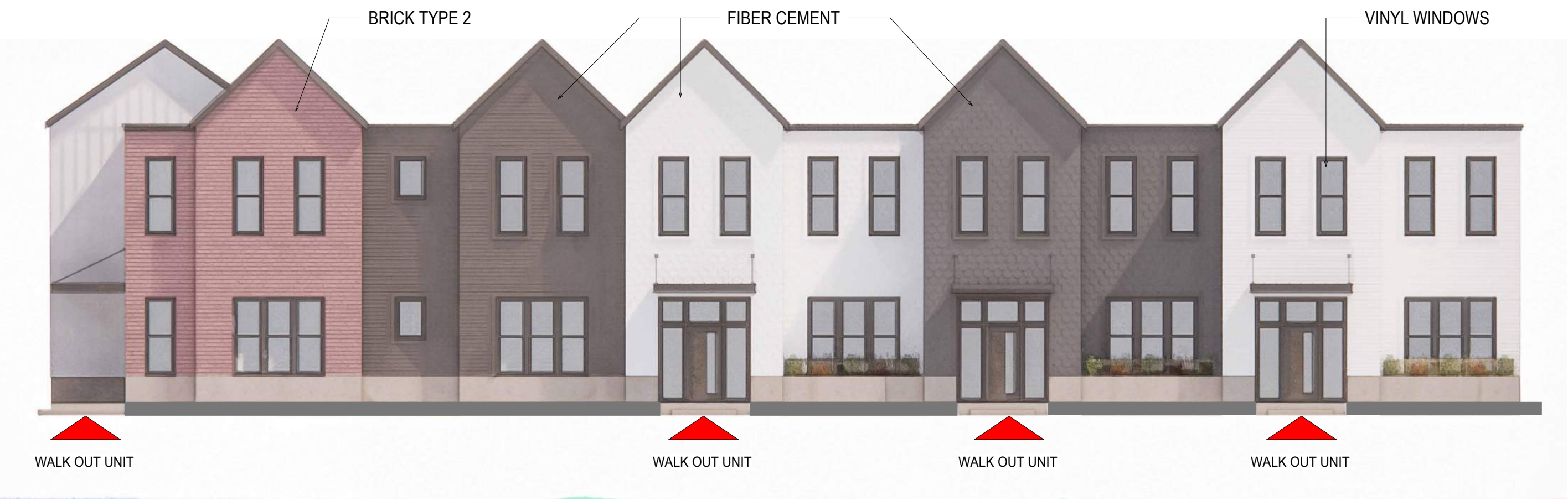
2 ELEVATION SOUTH ELEVATION - NORTHERN TOWNHOMES 1/8" = 1'-0" REF: 2 / 1
