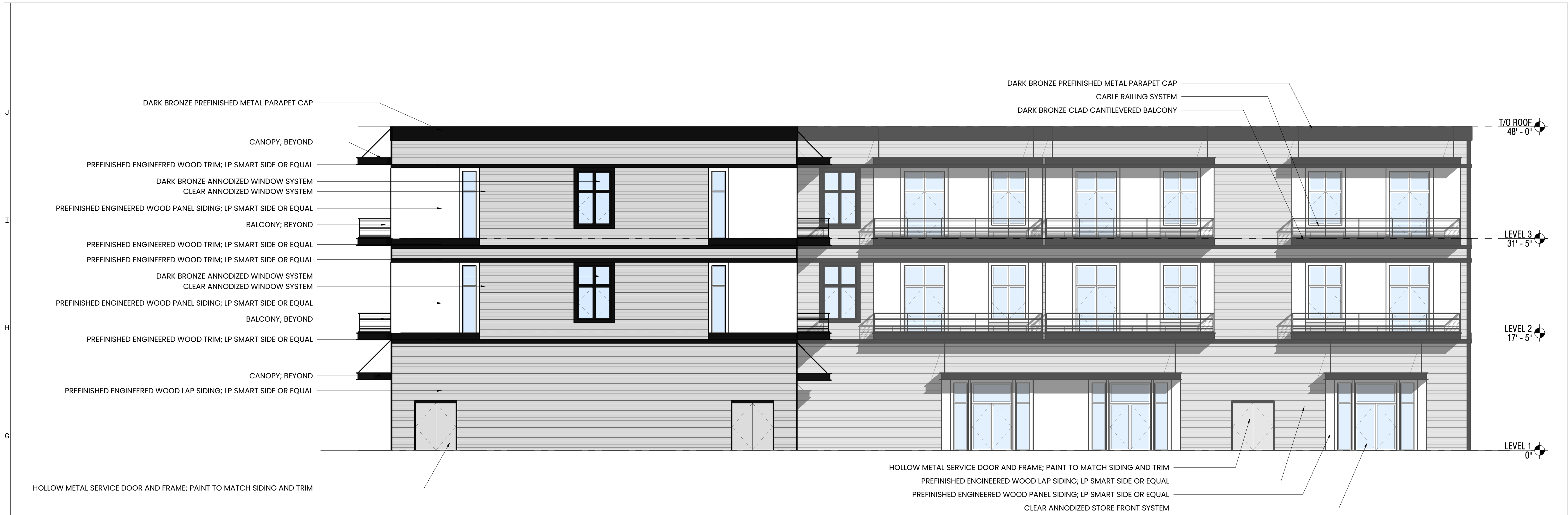
F1 East Elevation 1/8" = 1'-0" RE: A1/A101
