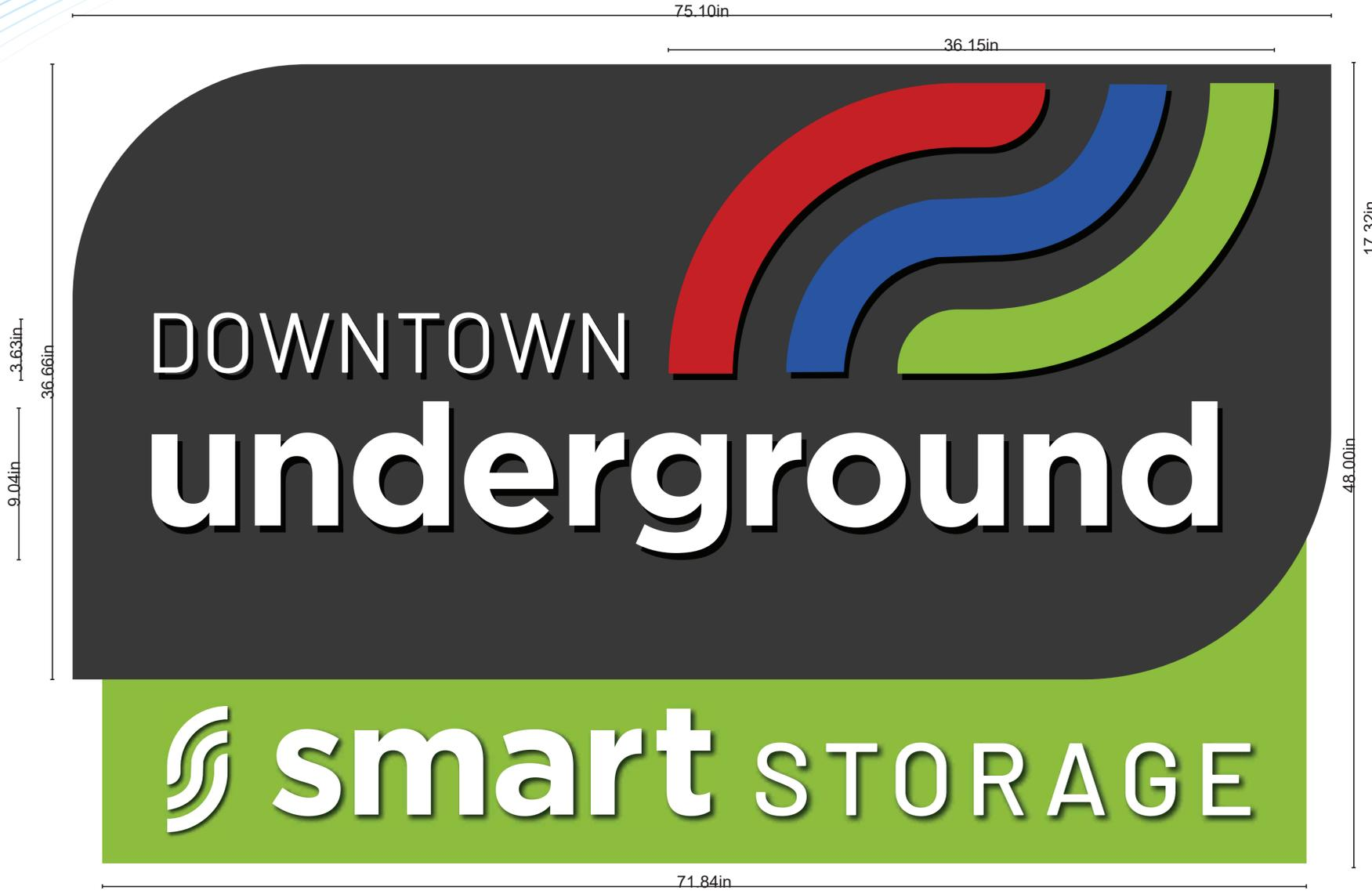
INTERNALLY LIT DOUBLE SIDED ROUTER CUT RADIUS CORNER CABINET
